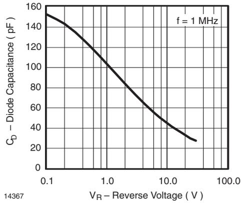
Fig. 5 - Typ. Diode Capacitance vs. Reverse Voltage
