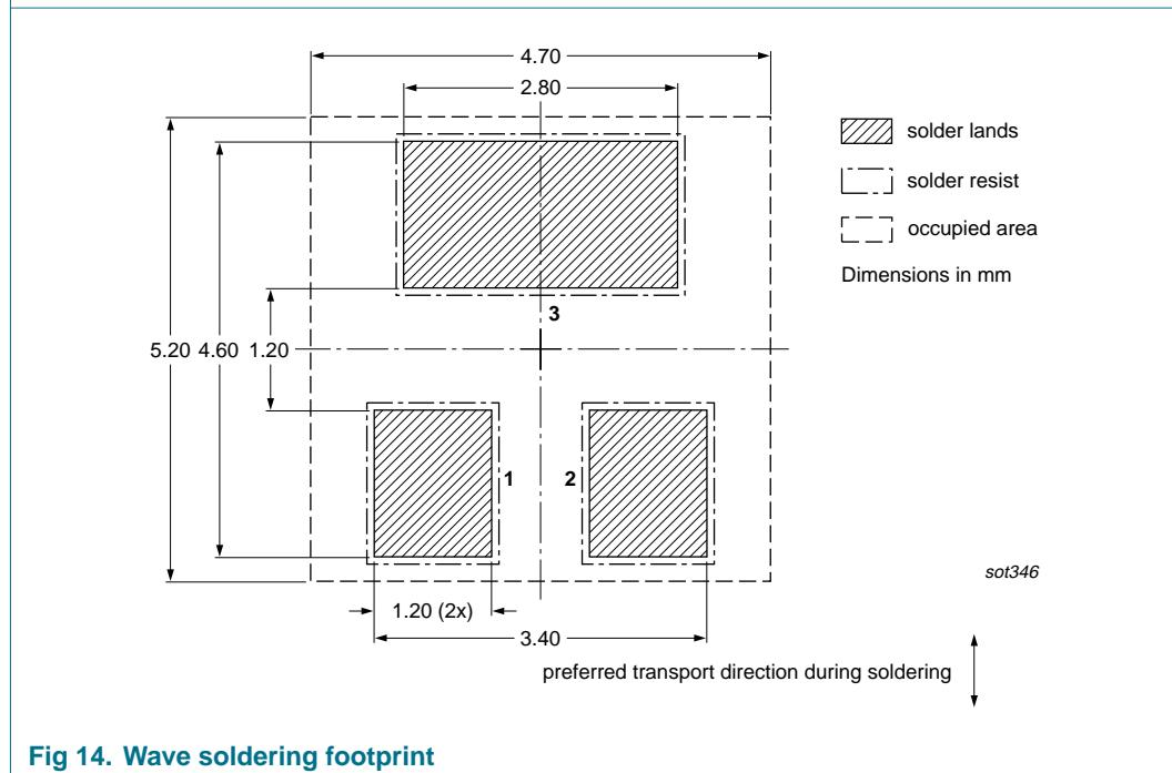
Fig 14. Wave soldering footprint
