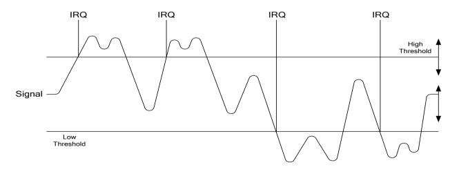
Figure 23 AuxADC IRQ Operation
