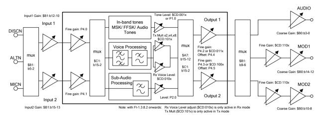
Figure 27 Level Adjustments
