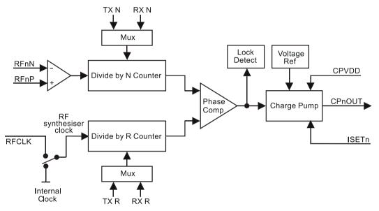
Figure 25 Single RF Channel Block Diagram
