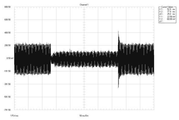
Figure 17 Compressor Transient Response
