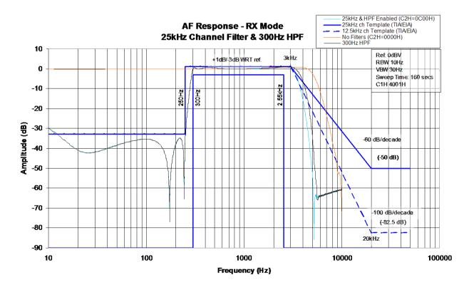
Figure 11 Rx 25kHz Channel Audio Filter Frequency Response
