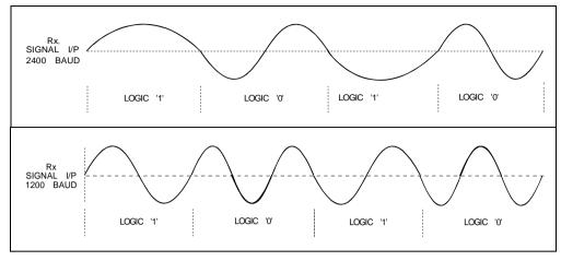
Figure 19 Modulating Waveforms for 1200 and 2400 Baud MSK/FFSK Signals
