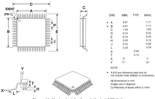
Figure 32 Mechanical Outline of 48-pin LQFP (L4)
