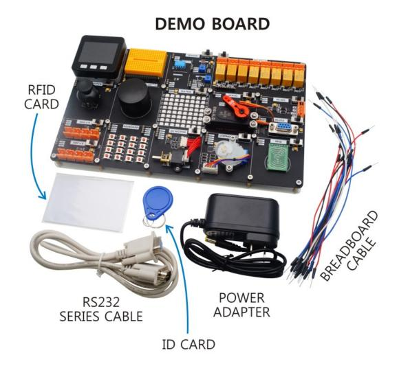
1x 12V power adapter (before using the development board, please connect the 12V power adapter to power the development board)
