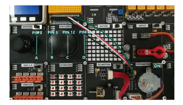
Different coil energization sequence will affect the rotation speed of the stepper motor, the number of beats for a complete revolution, the step value, and the stability during operation.
