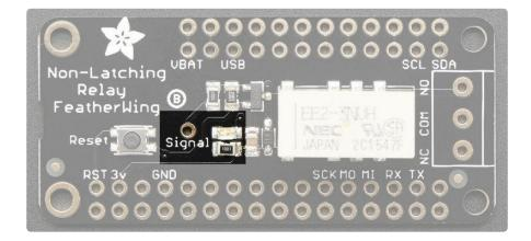
The plain relay uses a single pin for control. When the signal pin is floating or pulled low, the relay is 'open' or unset. When the signal pin is pulled high, the relay switches
