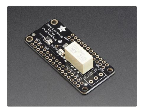
Both FeatherWings use the same family of relay. You can switch up to 2A of resistive current at 30VDC or ~40VAC or lower. At 110VDC you can switch up to 0.6A, at 120VAC up to 0.5A, and at 250VAC you can switch up to 0.3A. Check the datasheet for the relay for the exact switching capacity, and of course, for reactive/inductive loads you will need to derate. This isn't a relay you can use to turn on and off your washer/dryer, stick to 60W or less.
