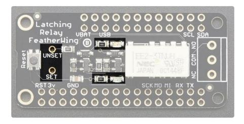
The latching relay uses two pins for control. There is no way to know which 'orientation' the relay is when the Feather turns on, because the relay will latch in the last position it was set to.
