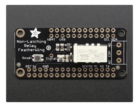
A Feather board without ambition is a Feather board without FeatherWings! These are the Mini Relay FeatherWing. They will give you power to control, and control over power. Put simply, you can now turn on and off lamps, fans, solenoids, and other small appliances that run on up to 250VAC or DC power using any Feather board.
