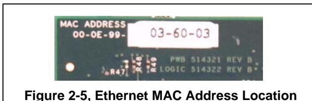
**Figure 2-5, Ethernet MAC Address Location**
