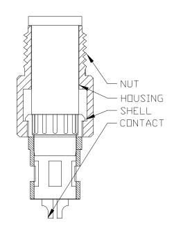
MATERIAL TPU, BLACK HOUSING: CONTACT: BRASS NUT: BRASS SHELL: BRASS FINISH CONTACT: GOLD PLATED □VER 50μ" NICKEL NUT: NICKEL PLATED SHELL: BRIGHT TIN PLATED ELECTRICAL RATED CURRENT: 1Α RATED VOLTAGE: 60V INSULATION RESISTANCE: 100 MOhms MIN.
