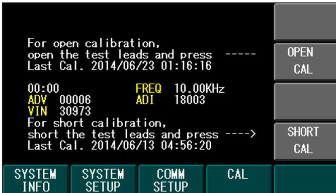
Figure 3.1 – Open Calibration
