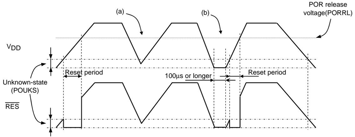
Figure 8 Waveform observed when only POR is used (LVD not used)
