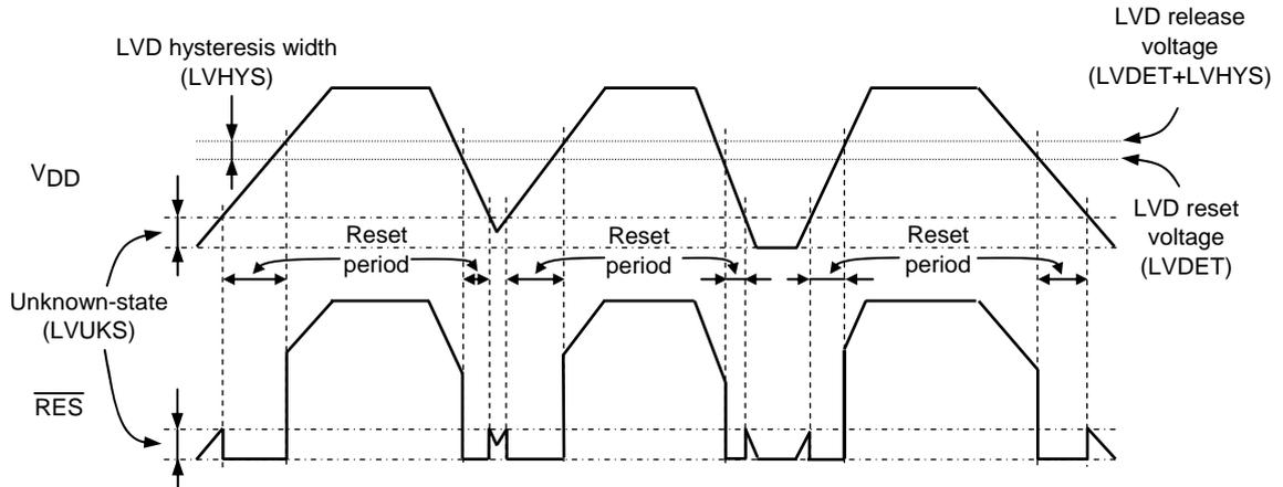
Figure 9 Waveform observed when both POR and LVD functions are used
