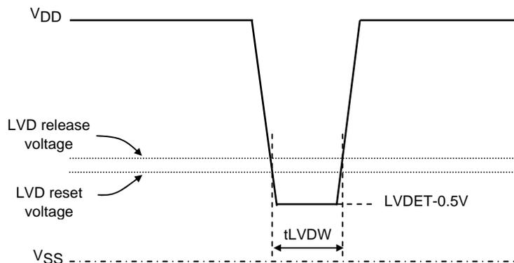
Figure 10 Low voltage detection minimum width
