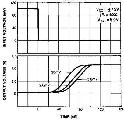
Figure 7. Response Time for Various Input Overdriver
