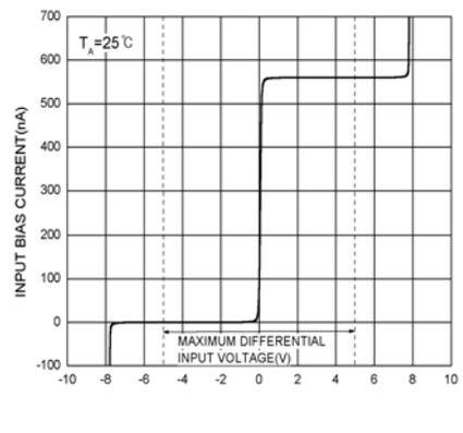
Figure 6. Input Characteristics
