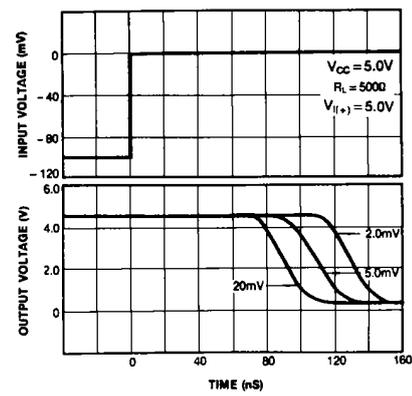
Figure 4. Response Time for Various Input Overdriver
