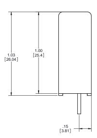
Tolerances: ± 0.02 in / 0.5 mm. All dimensions are in: inches [millimeters]
