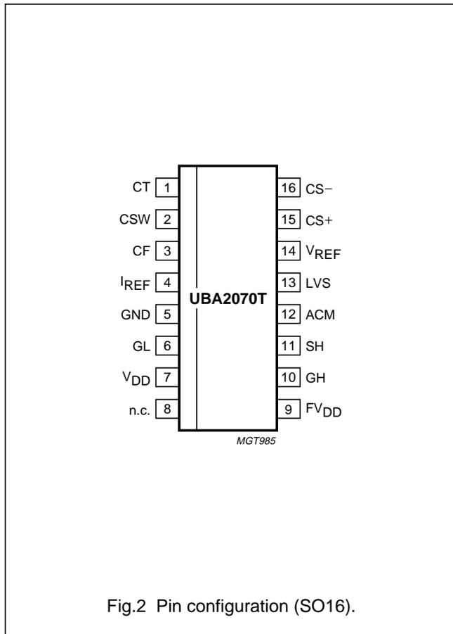
Fig.2 Pin configuration (SO16).
