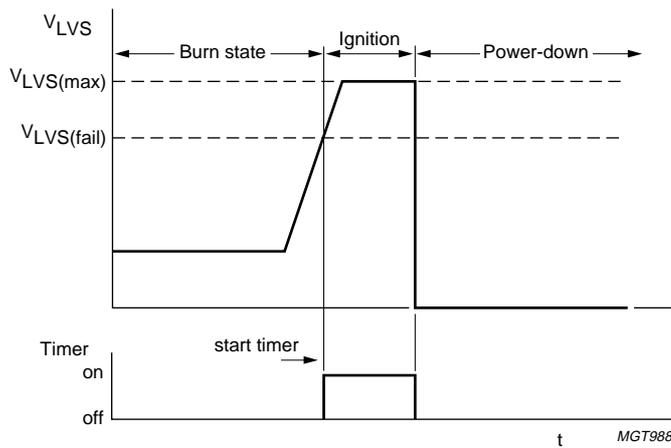
Fig.7 Lamp failure during burn state.
