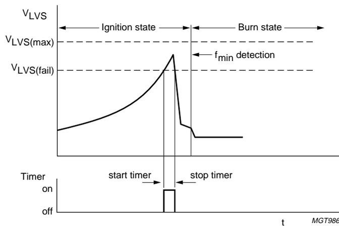
Fig.5 Normal ignition behaviour.
