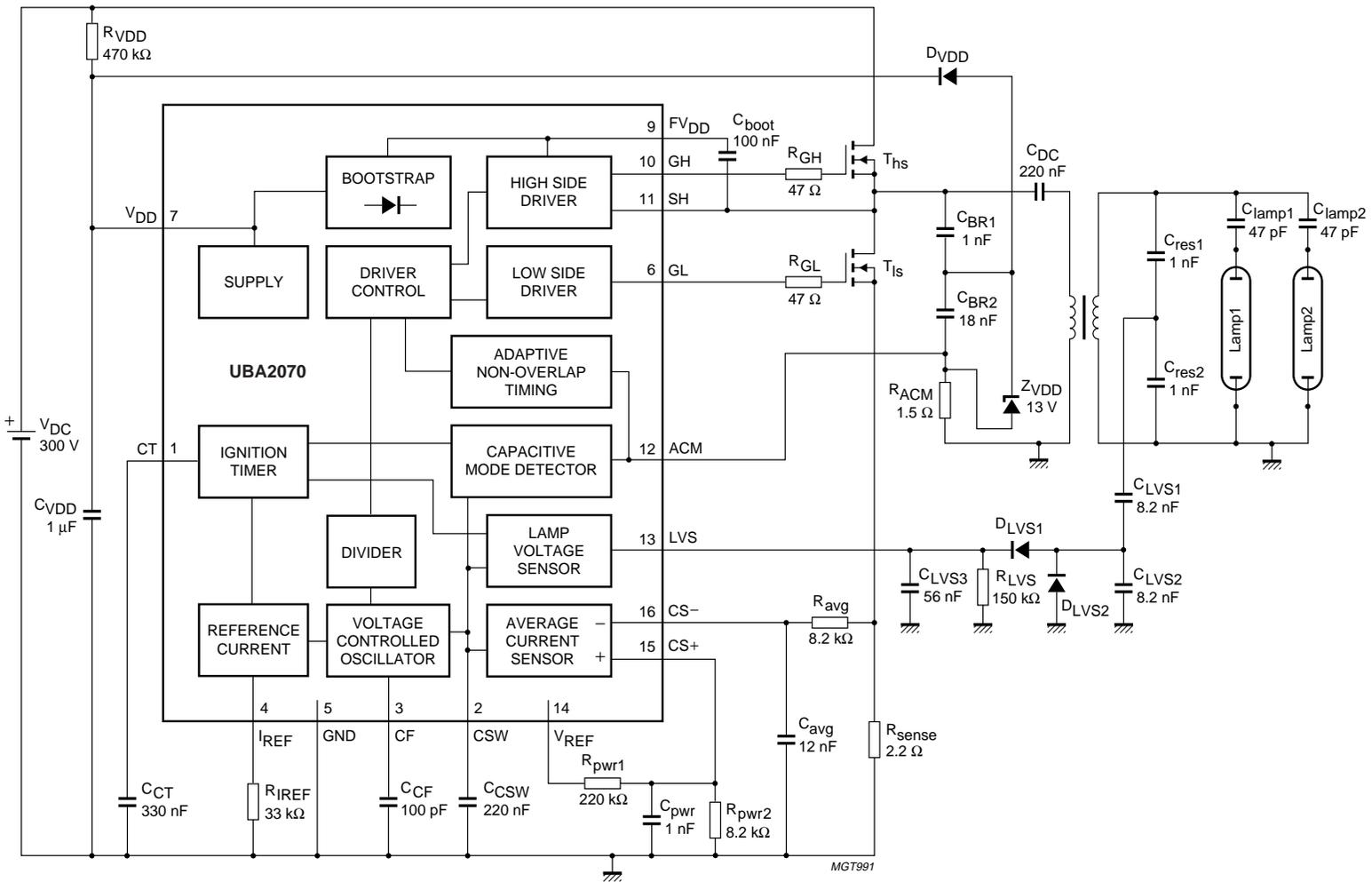
Fig.8 Test application circuit.
