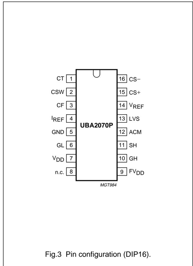
Fig.3 Pin configuration (DIP16).
