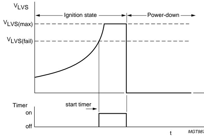
Fig.6 Lamp failure during ignition state.
