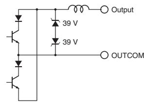
Note: Although the output terminals are electrically insulated from the internal circuit, do not conduct an insulation resistance test on these terminals.
