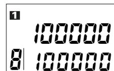
(2) Press the **RESET** Key (or turn ON the reset input) to reset the count value to 0 for that counter only.
