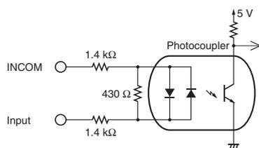
Note: Although the input terminals are electrically insulated from the internal circuit, do not conduct an insulation resistance test on these terminals.
