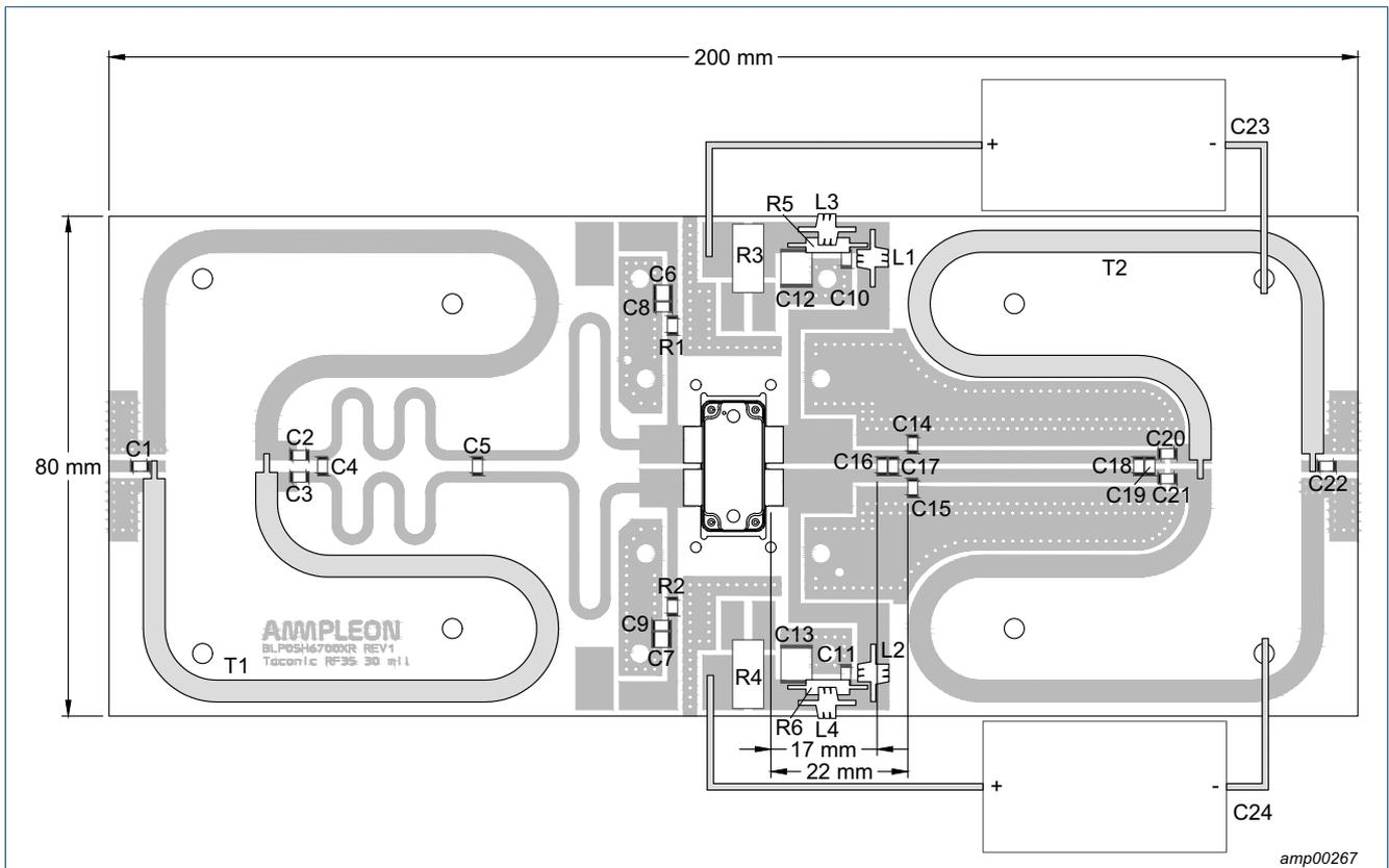
Printed-Circuit Board (PCB): Taconic RF-35;  $\epsilon_r = 3.5$  F/m; thickness = 0.765 mm; thickness copper plating = 35  $\mu$ m.
