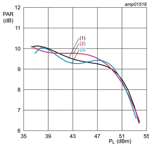
$V_{DS} = 48 \text{ V}; I_{Dq} = 820 \text{ mA}; V_{GS(amp)peak} = 0.25 \text{ V}.$
