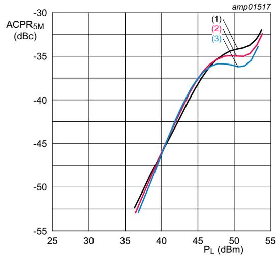
$V_{DS} = 48 \text{ V}; I_{Dq} = 820 \text{ mA}; V_{GS(amp)peak} = 0.25 \text{ V}.$
