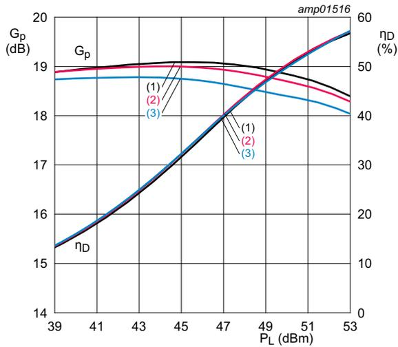
$V_{DS} = 48 \text{ V}; I_{Dq} = 820 \text{ mA}; V_{GS(amp)peak} = 0.25 \text{ V}.$
