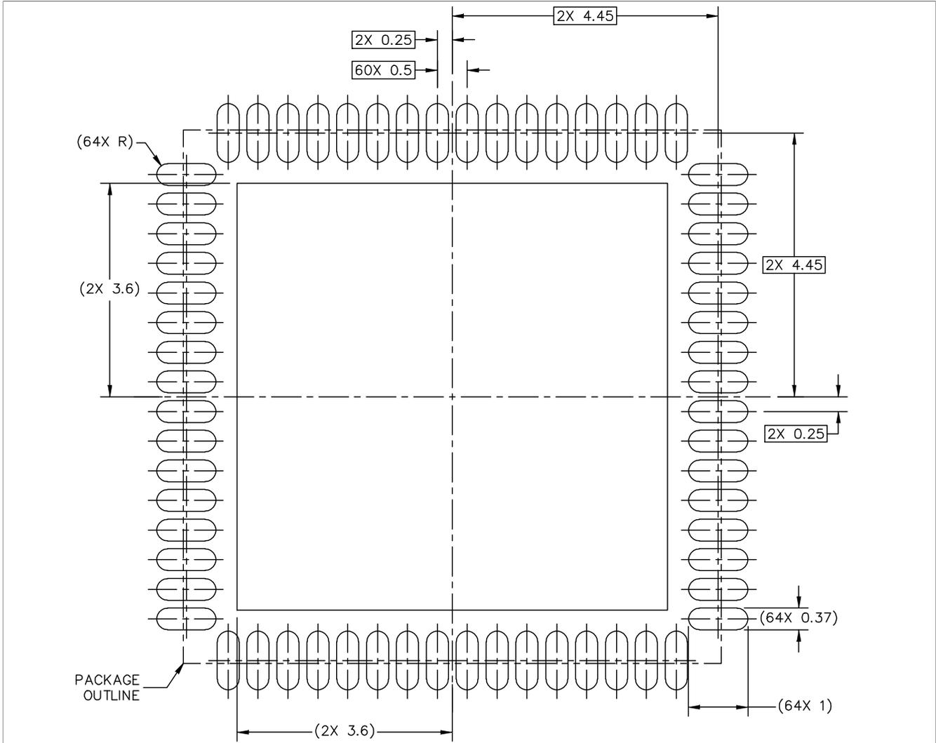
PCB DESIGN GUIDELINES – SOLDER MASK OPENING PATTERN
