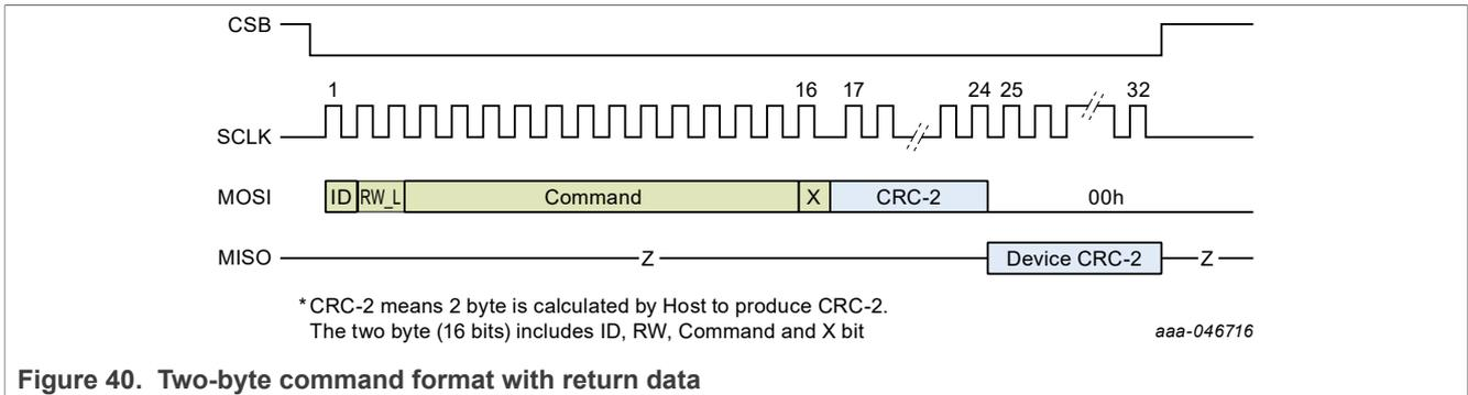
Figure 40. Two-byte command format with return data
