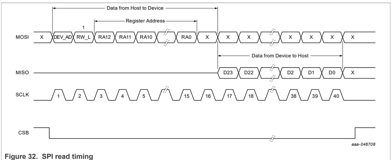
Figure 32. SPI read timing
