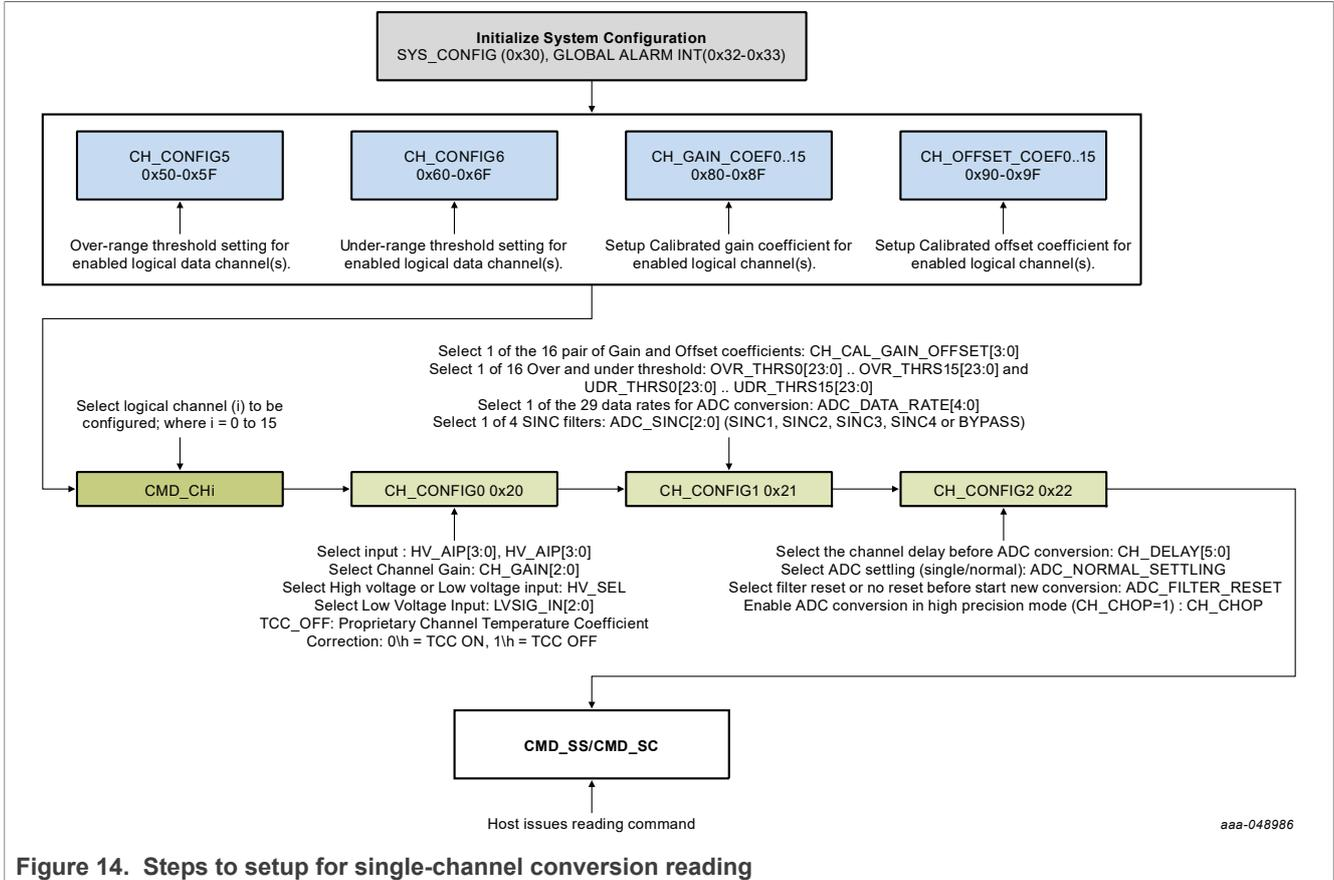
Figure 14. Steps to setup for single-channel conversion reading
