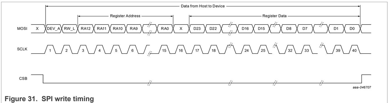
Figure 31. SPI write timing
