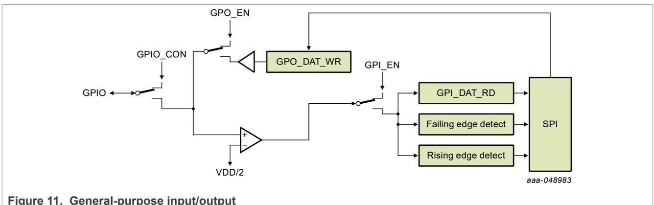
Figure 11. General-purpose input/output
