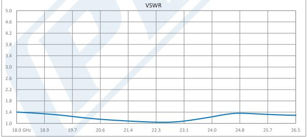
Click the following link (or enter part number in "SEARCH" on website) to obtain additional part information including price, inventory and certifications: Isolator with 14 dB Isolation from 18 GHz to 26.5 GHz, Hermetically Sealed, 10 Watts and 2.92mm Female PE83IR1041
