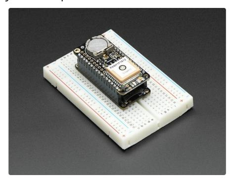
The GPS has a built in real time clock, which can keep track of time even when it power is lost and it doesn't have a fix yet. It can also help reduce fix times, if you
