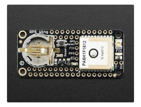
Give your Feather a sense of place, with an Ultimate GPS FeatherWing. This FeatherWing plugs right into your Feather board and gives it a precise, sensitive, and low power GPS module for location identification anywhere in the world. As a bonus, the GPS can also keep track of time once it is synced with the satellites.
