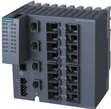
SCALANCE XC216-4C manageable Layer 2 IE switch; IEC 62443-4-2 certified; 12x 10/100 Mbit/s RJ45 ports; 4x 1000 Mbit/s combo ports (either 1000 Mbit/s/ SFPs or 10/100/1000 Mbit/s RJ45 ports can be used); 1x console port; diagnostics LED; redundant power supply; temperature range -40 °C to +70 °C; assembly: DIN rail/S7 mounting rail/wall; redundancy functions; office features (RSTP, VLAN,...); PROFINET IO device; Ethernet/IP-compliant; C-PLUG slot;
