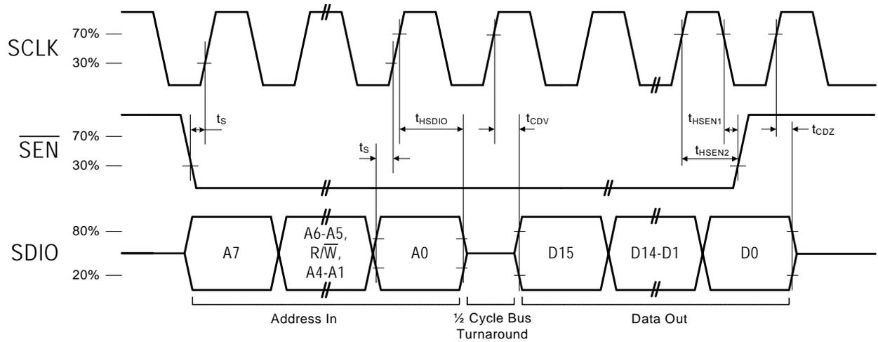
Figure 4. 3-Wire Control Interface Read Timing Parameters
