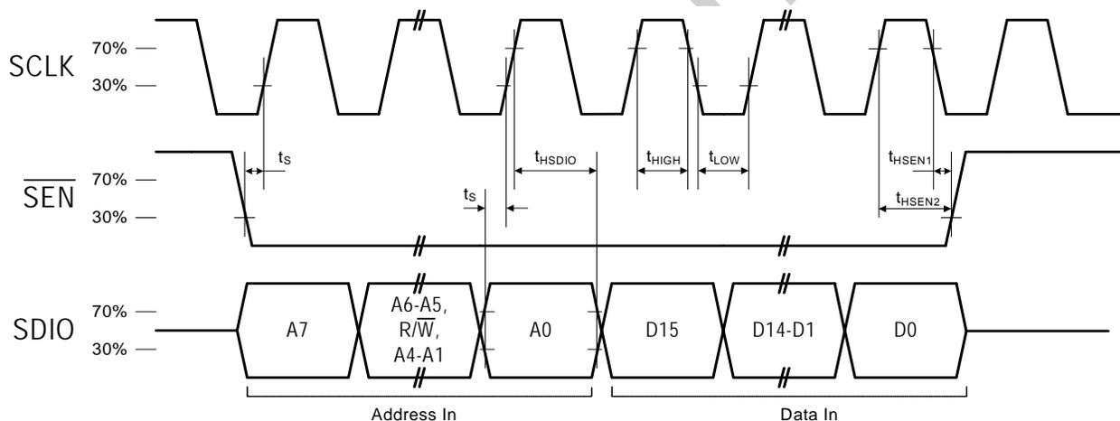
**Figure 3. 3-Wire Control Interface Write Timing Parameters**
