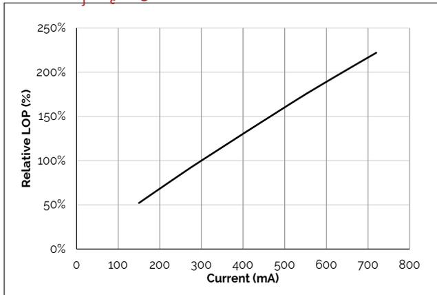
**Figure 4: V8E Typical Relative Luminous Flux vs. Drive Current ( $T_j = T_c = 25^\circ\text{C}$ )<sup>1</sup>**
