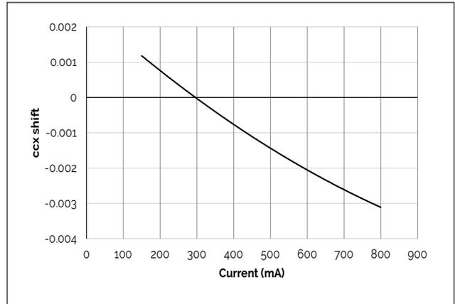
**Figure 9: V8D Drive Current vs. ccy Shift**
