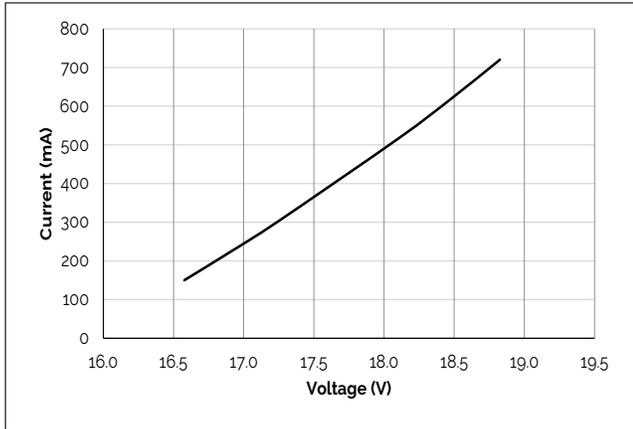
**Figure 2: V8E Drive Current vs. Voltage ( $T_j = T_c = 25^\circ\text{C}$ )<sup>1</sup>**
