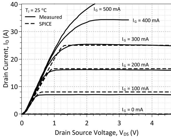
**Figure 1: Typical Output Characteristics at 25 °C**
