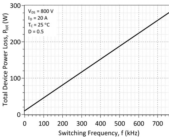
**Figure 15: Typical Hard Switched Device Power Loss vs. Switching Frequency<sup>2</sup>**
