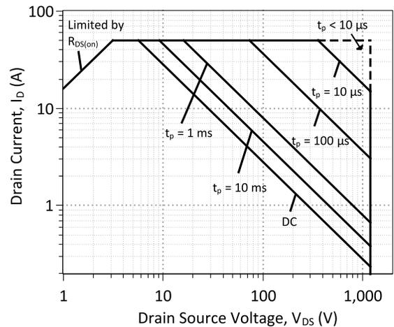
**Figure 18: Forward Bias Safe Operating Area at T<sub>c</sub> = 25 °C**
