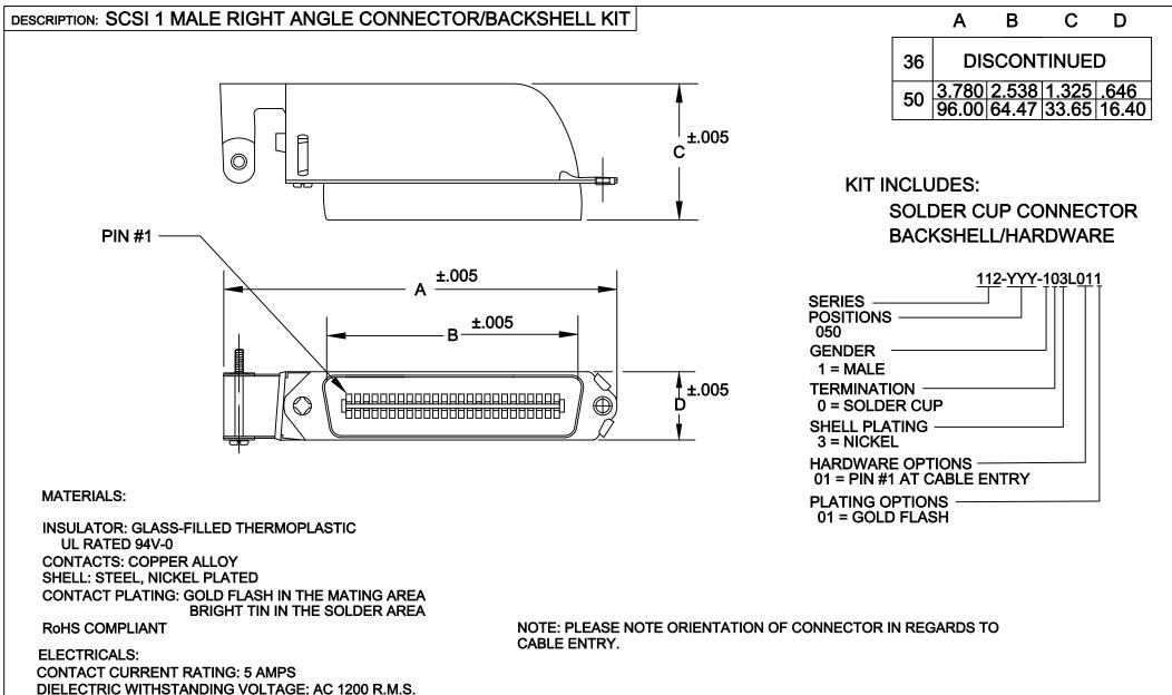
INSULATION RESISTANCE: 1000 mohms MINIMUM AT 500V DC
