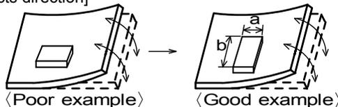
Products shall be located in the sideways direction (Length:a < b) to the mechanical stress.
