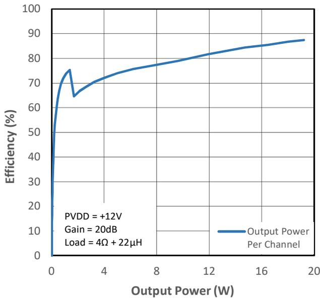
Figure 14-11 PMP2 Efficiency (VDD+PVDD) vs Output Power
