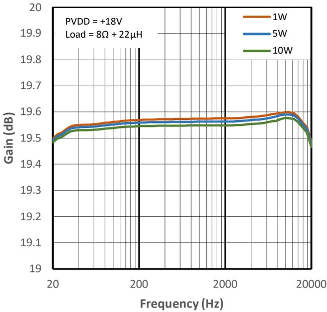
Figure 11-25 Low Gain vs Frequency for PMP0
