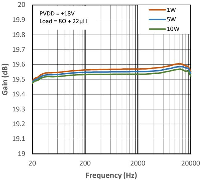
Figure 11-27 Low Gain vs Frequency for PMP2
