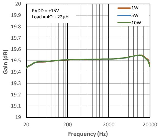
Figure 12-24 Low Gain vs Frequency for PMP4
