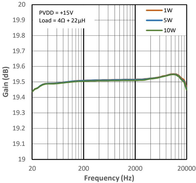
Figure 12-21 Low Gain vs Frequency for PMP0
