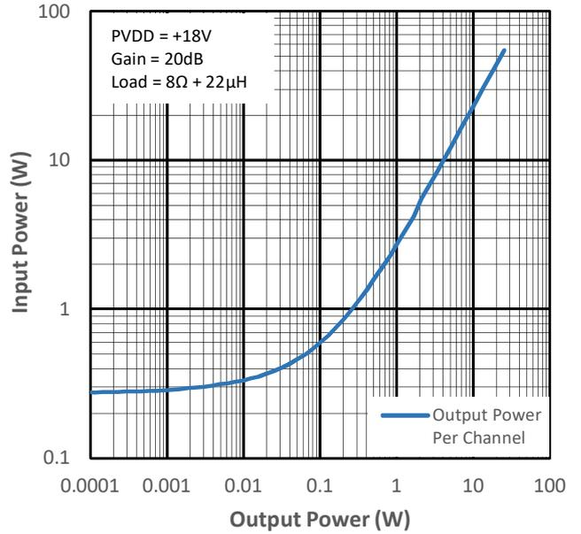
Figure 11-14 Input Power vs Output Power for PMP1
