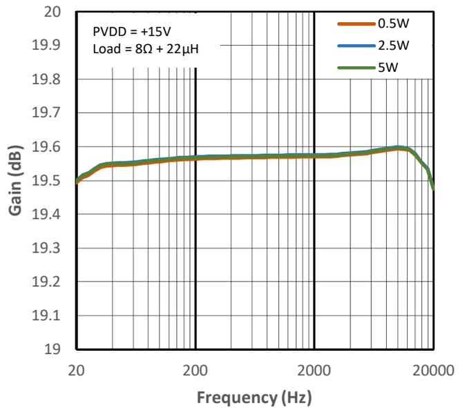
Figure 13-24 Low Gain vs Frequency for PMP4
