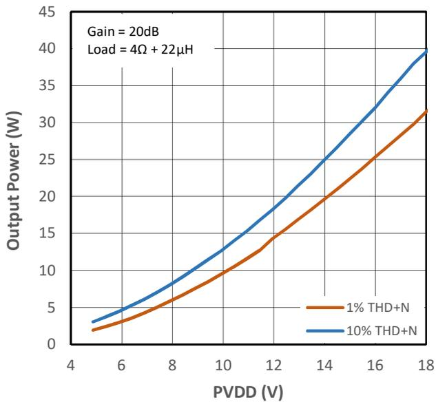
Figure 10-23 Output Power vs PVDD Voltage for PMP2
