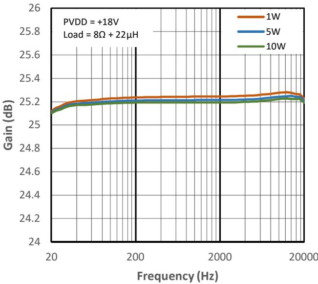
Figure 11-31 High Gain vs Frequency for PMP2
