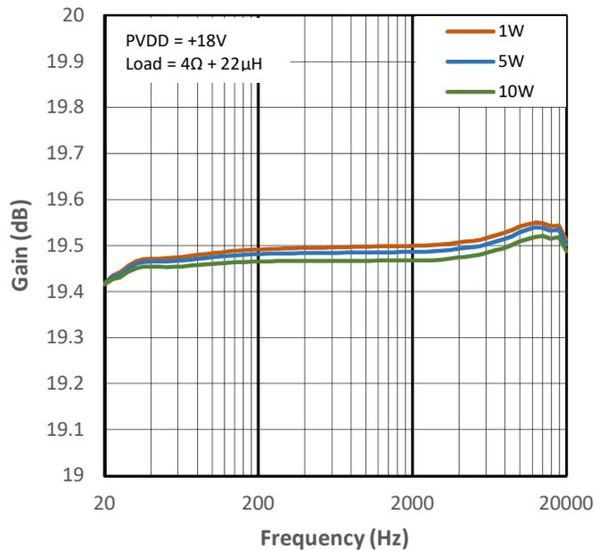
**Figure 10-26 Low Gain vs Frequency for PMP1**
