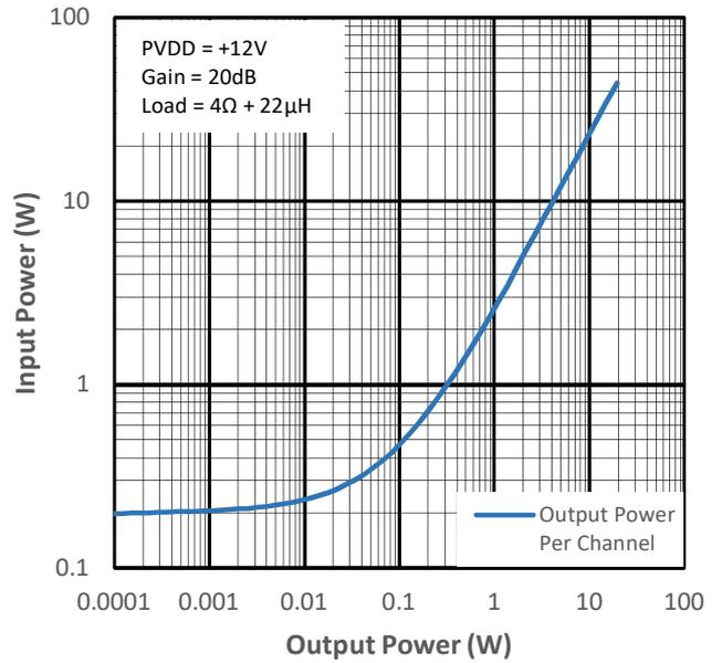
Figure 14-16 Input Power vs Output Power for PMP4
