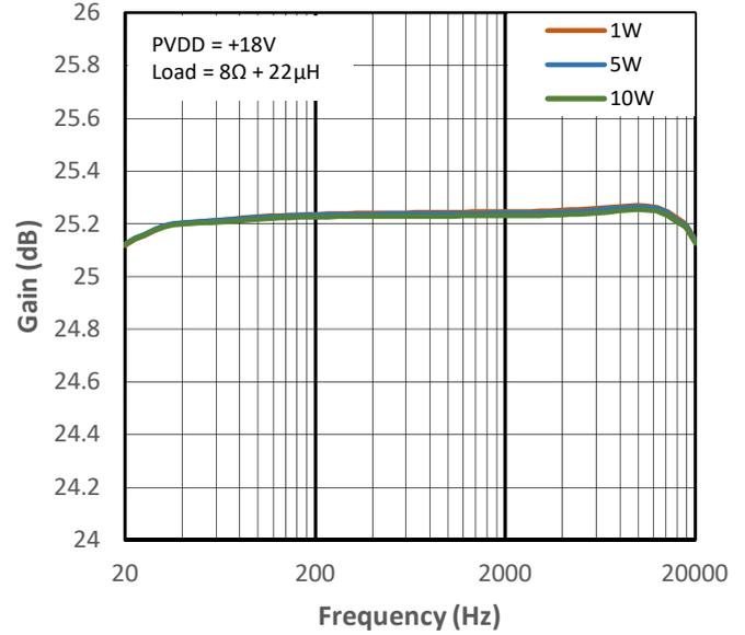
Figure 11-32 High Gain vs Frequency for PMP4
