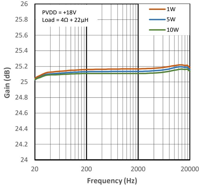
**Figure 10-30 High Gain vs Frequency for PMP1**
