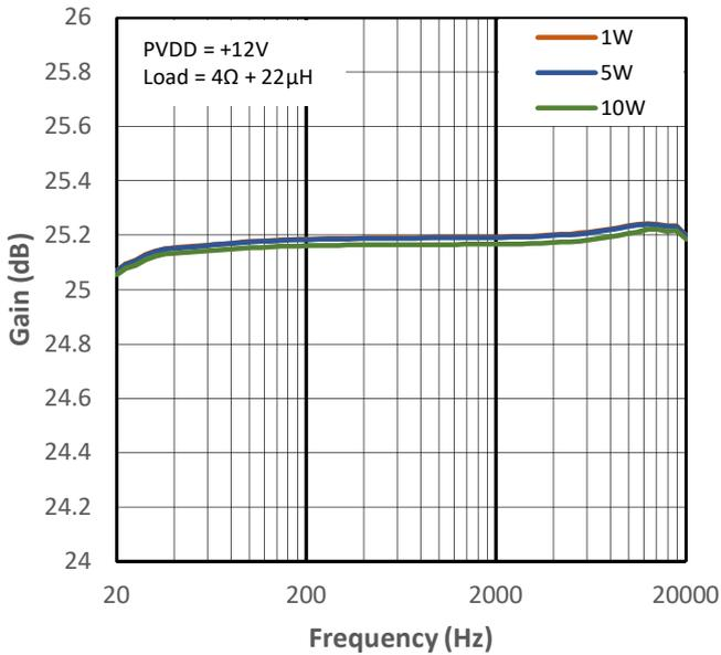
Figure 14-27 High Gain vs Frequency for PMP2
