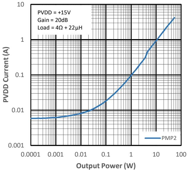
Figure 12-19 PVDD Current vs Output Power for PMP2
