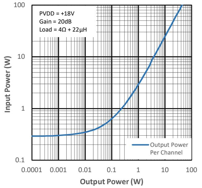
Figure 10-14 Input Power vs Output Power for PMP1
