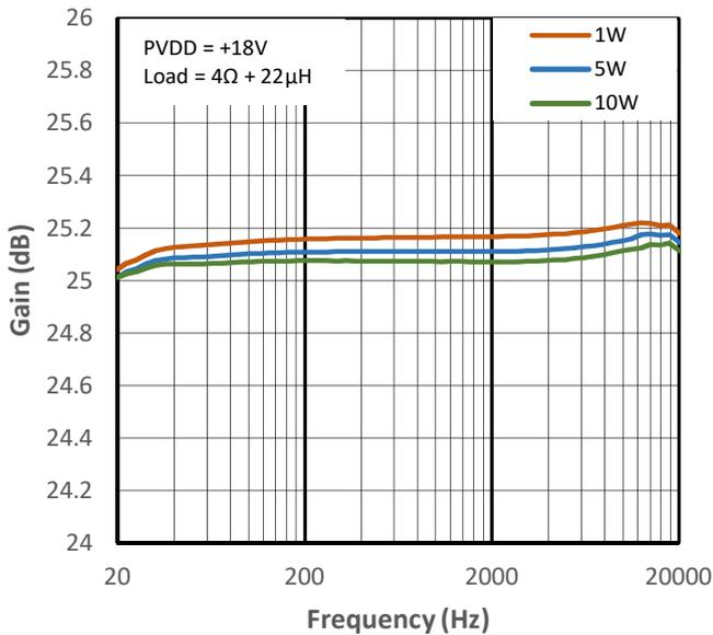
**Figure 10-31 High Gain vs Frequency for PMP2**
