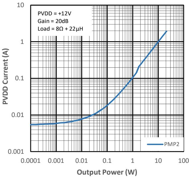
Figure 15-19 PVDD Current vs Output Power for PMP2
