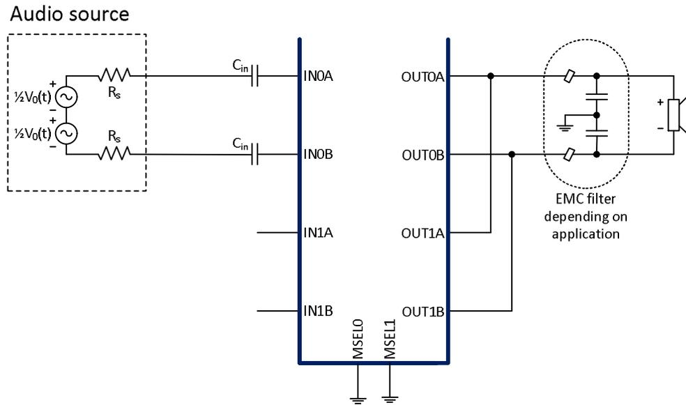
Figure 9-5 Parallel Bridge Tied Load (PBTL) configuration
