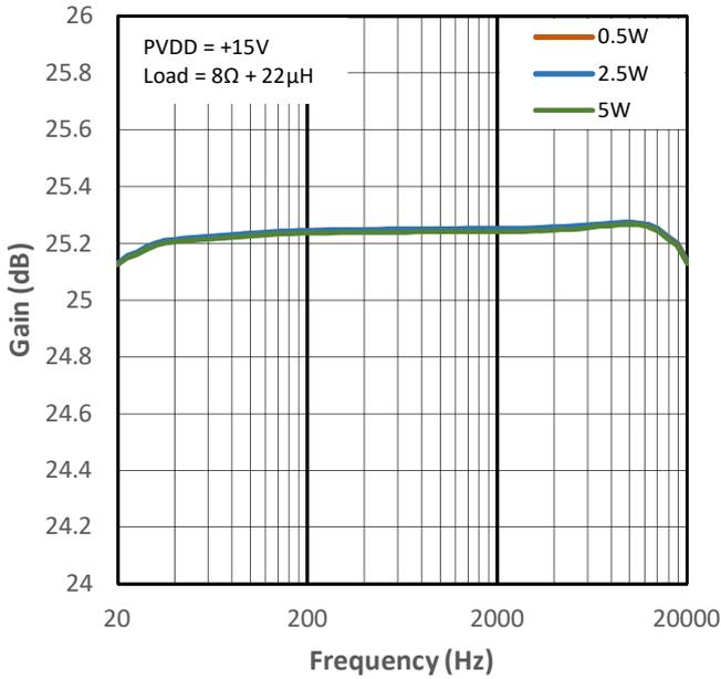
Figure 13-25 High Gain vs Frequency for PMP0
