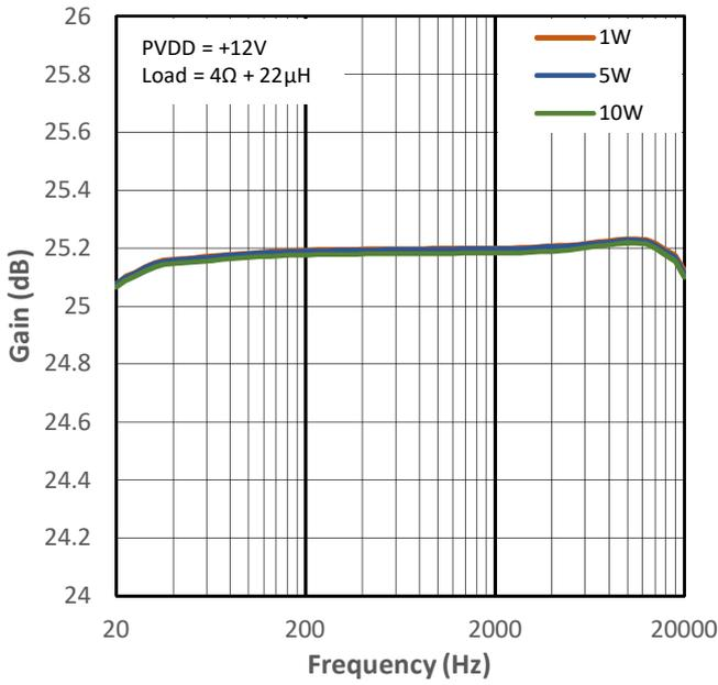
Figure 14-25 High Gain vs Frequency for PMP0
