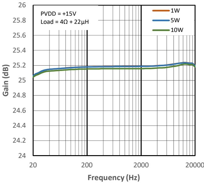
Figure 12-27 High Gain vs Frequency for PMP2
