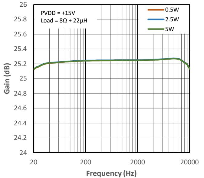
Figure 13-28 High Gain vs Frequency for PMP4
