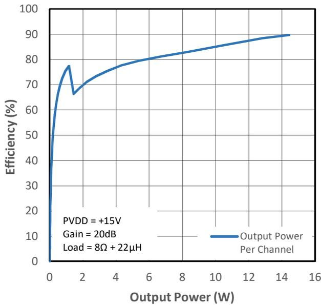
Figure 13-11 PMP2 Efficiency (VDD+PVDD) vs Output Power
