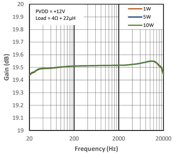
**Figure 14-24 Low Gain vs Frequency for PMP4**
