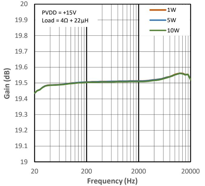
Figure 12-22 Low Gain vs Frequency for PMP1
