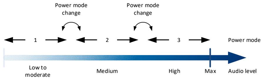
**Figure 8-1 Illustration of automatic power mode selection ranges**
