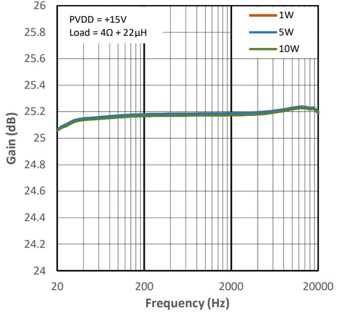
Figure 12-26 High Gain vs Frequency for PMP1
