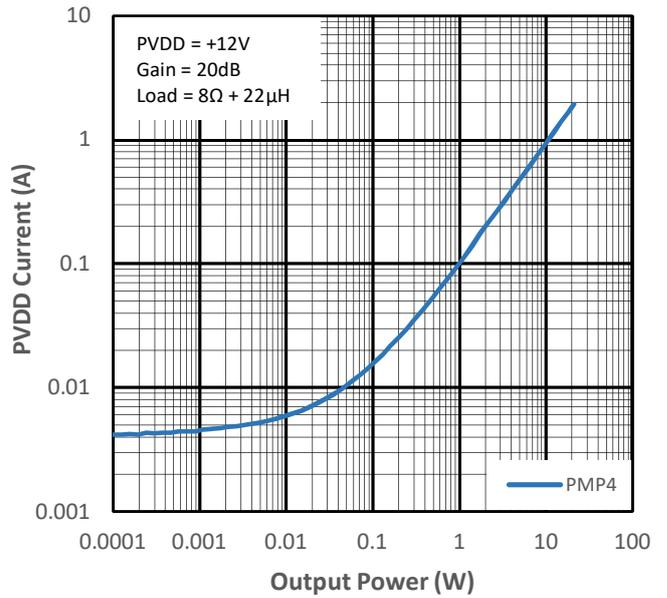
Figure 15-20 PVDD Current vs Output Power for PMP4
