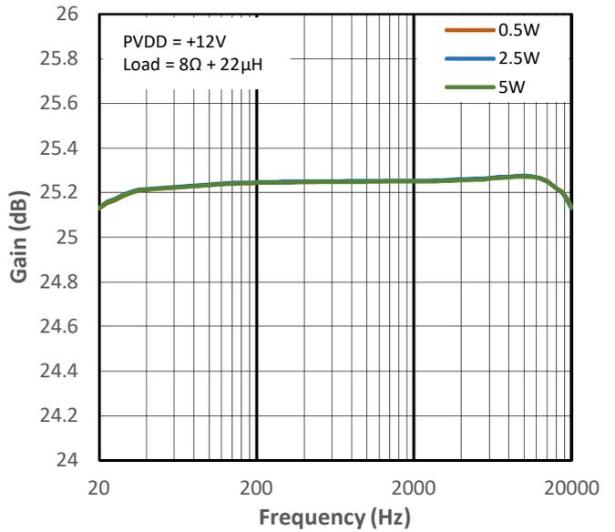
**Figure 15-28 High Gain vs Frequency for PMP4**
