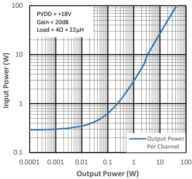
Figure 10-15 Input Power vs Output Power for PMP2
