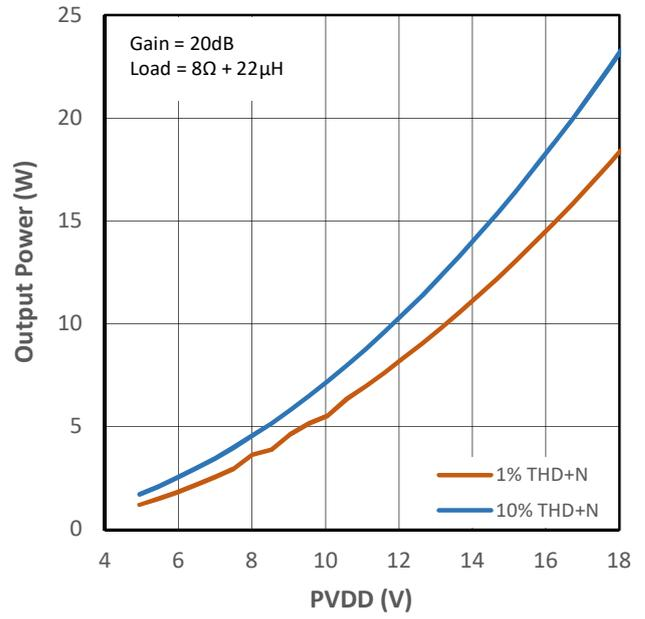
Figure 11-22 Output Power vs PVDD Voltage for PMP1
