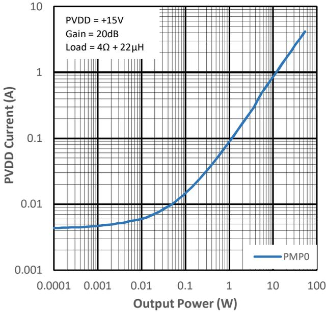
Figure 12-17 PVDD Current vs Output Power for PMP0
