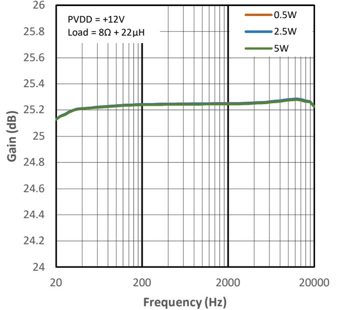
**Figure 15-26 High Gain vs Frequency for PMP1**
