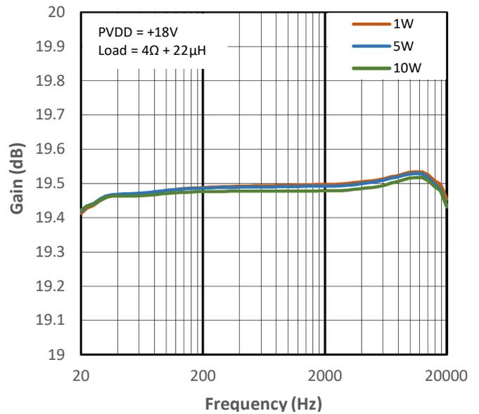
**Figure 10-28 Low Gain vs Frequency for PMP4**
