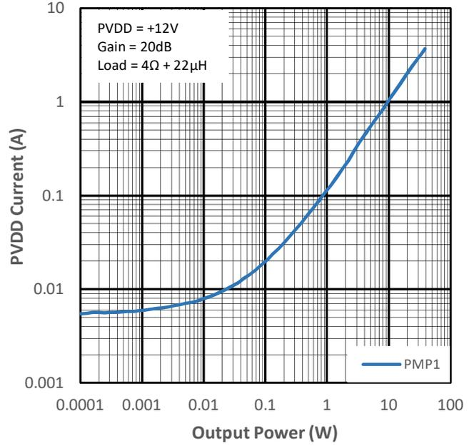
Figure 14-18 PVDD Current vs Output Power for PMP1
