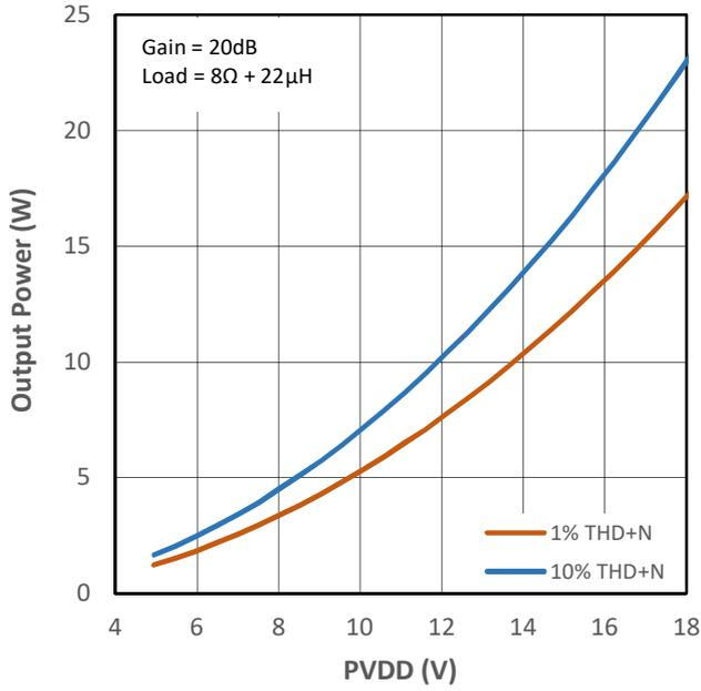
Figure 11-21 Output Power vs PVDD Voltage for PMP0
