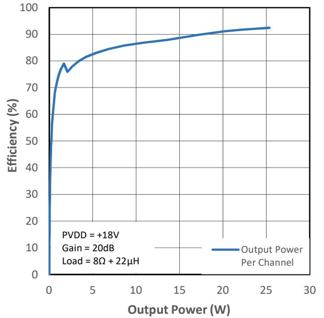
Figure 11-10 PMP1 Efficiency (VDD+PVDD) vs Output Power
