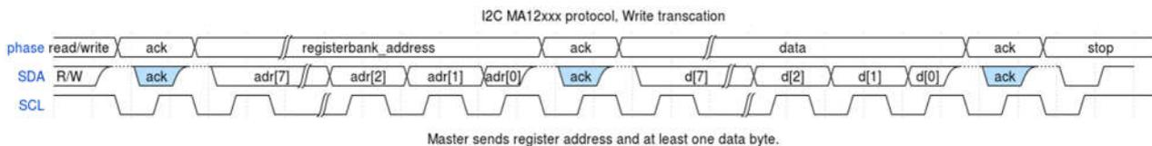
Figure 8-4 I2C write operation
