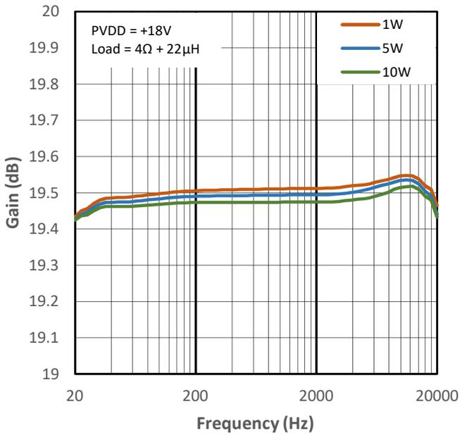
**Figure 10-25 Low Gain vs Frequency for PMP0**
