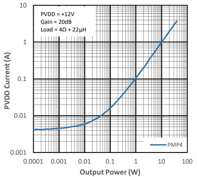
Figure 14-20 PVDD Current vs Output Power for PMP4
