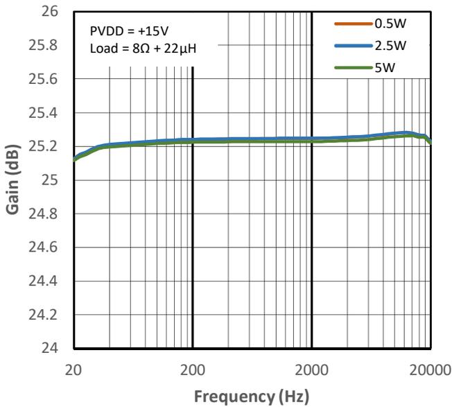
Figure 13-27 High Gain vs Frequency for PMP2
