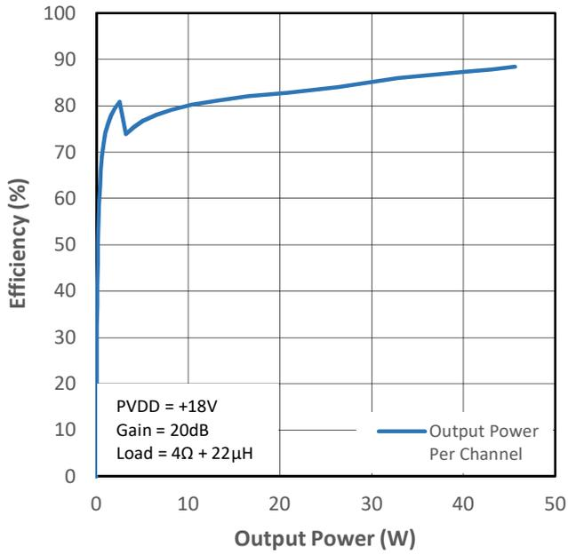
Figure 10-9 PMP0 Efficiency (VDD+PVDD) vs Output Power
