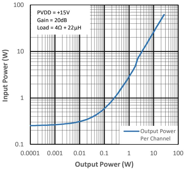
Figure 12-15 Input Power vs Output Power for PMP2
