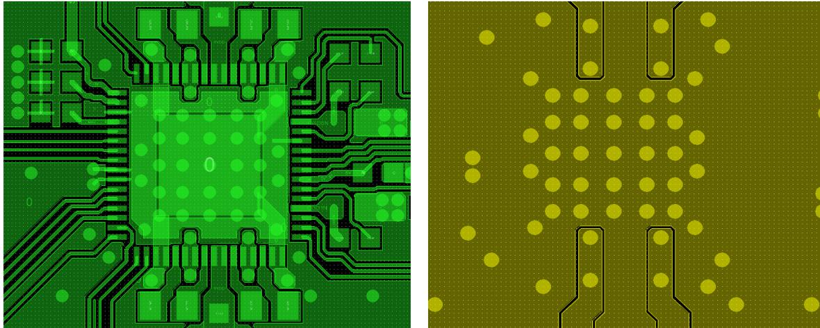
It is recommended to use a PCB made from glass/epoxy laminate (e.g. FR-4) material. This type of material works well with PCB designs that require thermal relief as it can endure high temperatures for a long duration of time.
