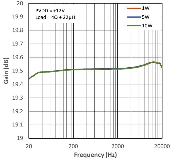
**Figure 14-22 Low Gain vs Frequency for PMP1**
