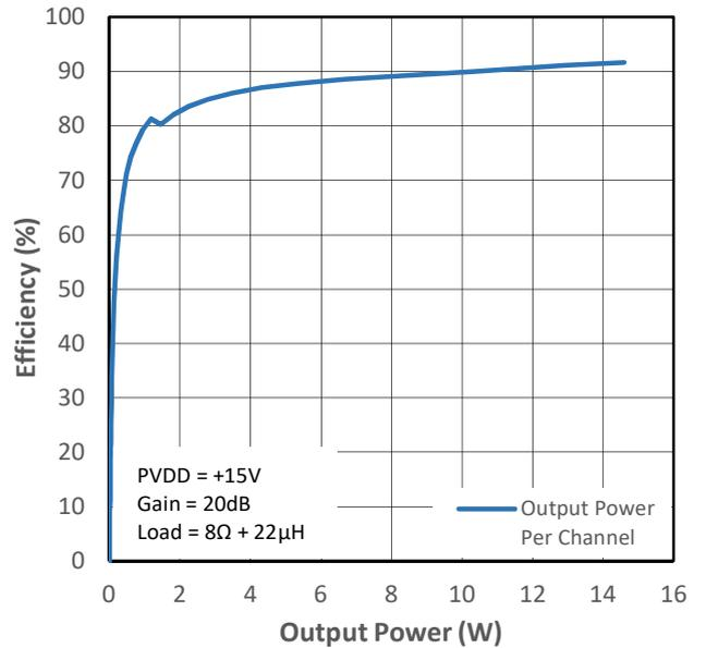
Figure 13-12 PMP4 Efficiency (VDD+PVDD) vs Output Power
