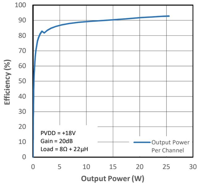
Figure 11-12 PMP4 Efficiency (VDD+PVDD) vs Output Power
