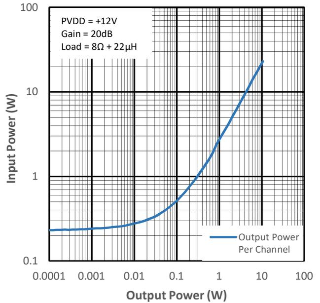
Figure 15-14 Input Power vs Output Power for PMP1
