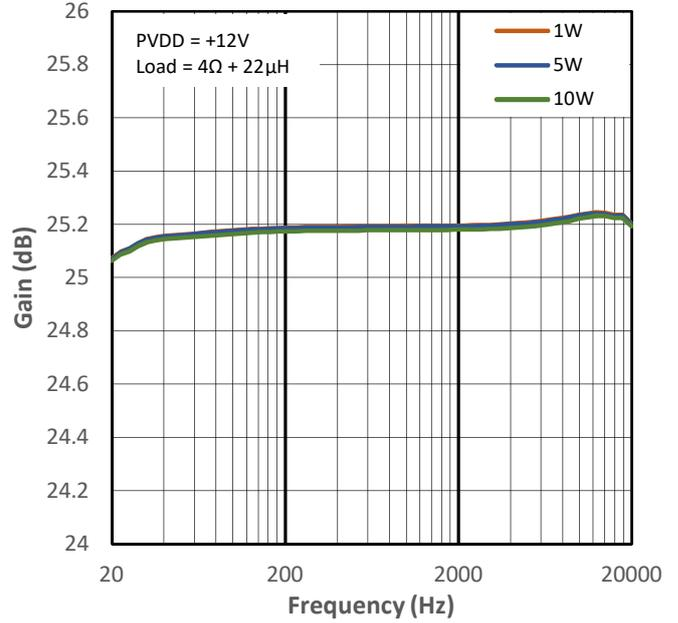
Figure 14-26 High Gain vs Frequency for PMP1
