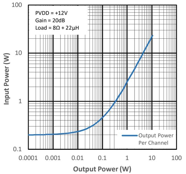
Figure 15-16 Input Power vs Output Power for PMP4
