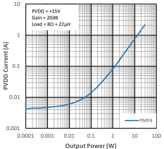
Figure 13-20 PVDD Current vs Output Power for PMP4
