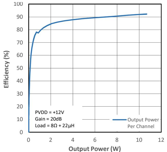
Figure 15-12 PMP4 Efficiency (VDD+PVDD) vs Output Power
