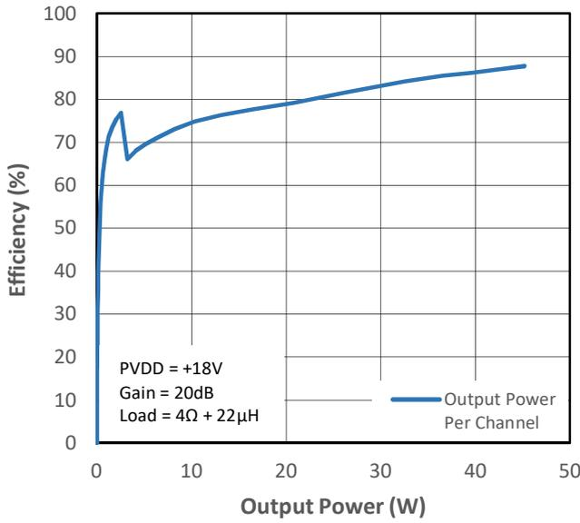
Figure 10-11 PMP2 Efficiency (VDD+PVDD) vs Output Power
