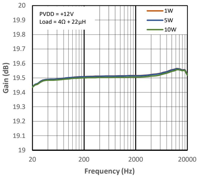
**Figure 14-23 Low Gain vs Frequency for PMP2**
