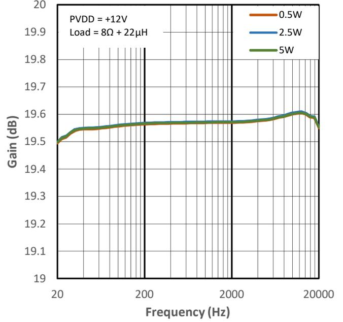
Figure 15-22 Low Gain vs Frequency for PMP1
