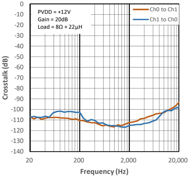
Figure 15-29 Crosstalk vs Frequency for PMP0
