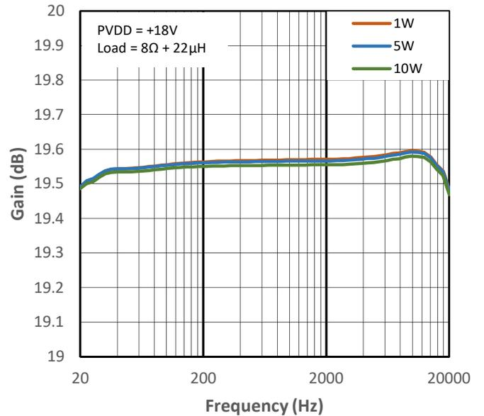
Figure 11-28 Low Gain vs Frequency for PMP4
