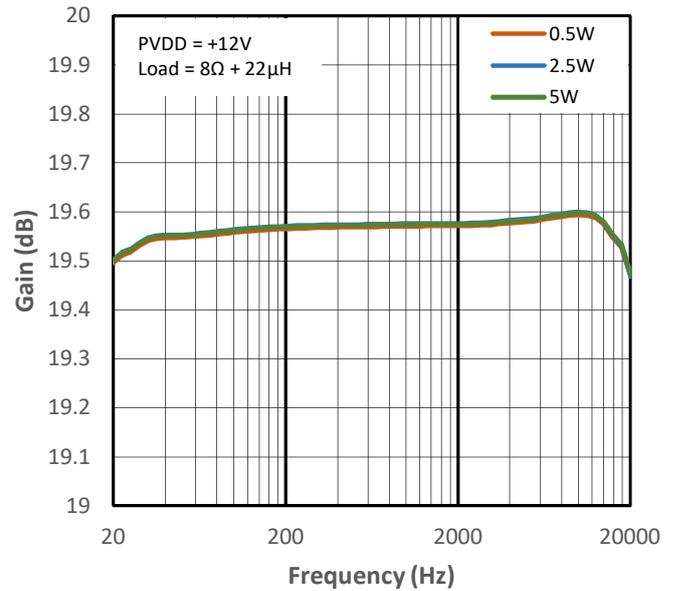
Figure 15-24 Low Gain vs Frequency for PMP4
