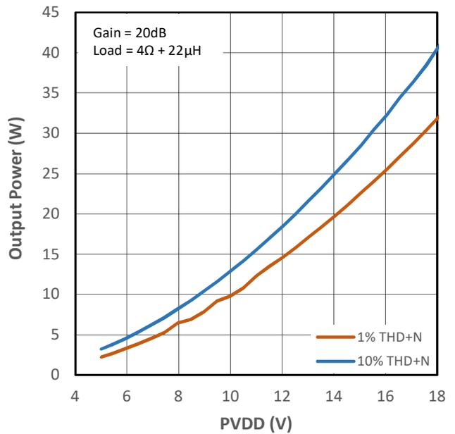
Figure 10-22 Output Power vs PVDD Voltage for PMP1
