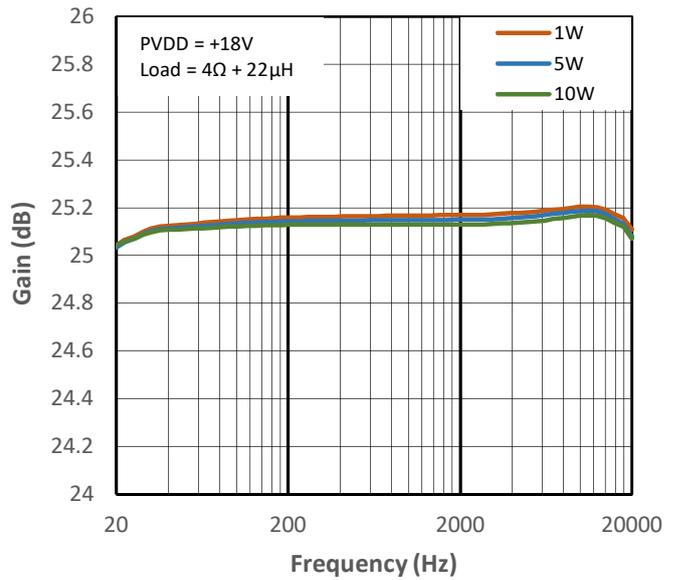
**Figure 10-32 High Gain vs Frequency for PMP4**
