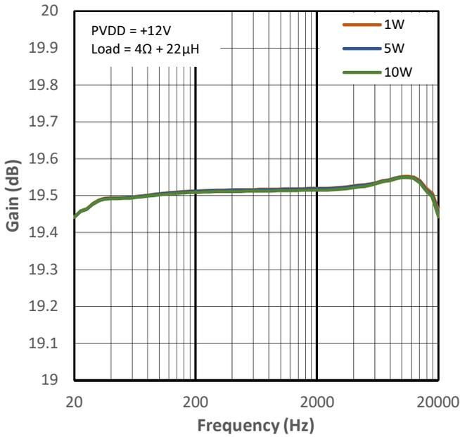
**Figure 14-21 Low Gain vs Frequency for PMP0**
