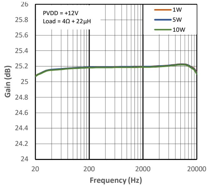
Figure 14-28 High Gain vs Frequency for PMP4
