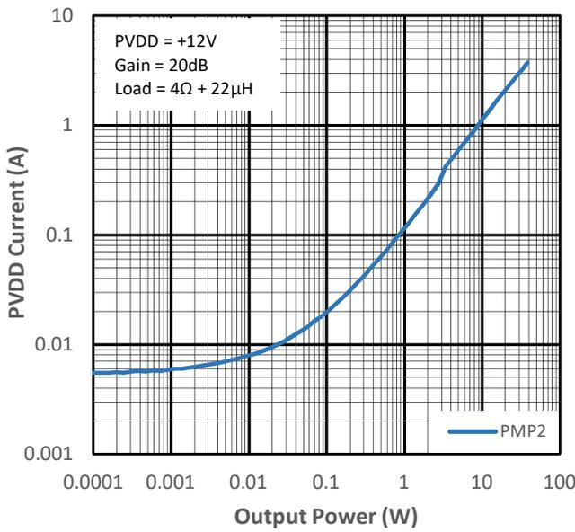
Figure 14-19 PVDD Current vs Output Power for PMP2
