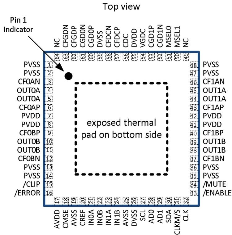
Figure 4-1 Pinout MA12040QFN
