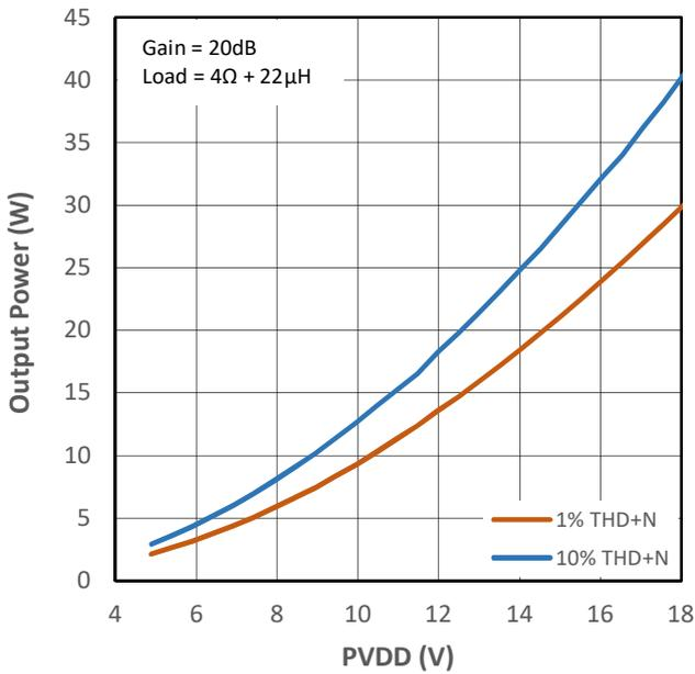
Figure 10-21 Output Power vs PVDD Voltage for PMP0
