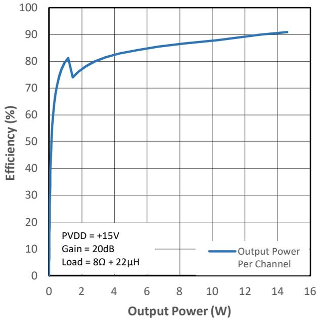
Figure 13-9 PMP0 Efficiency (VDD+PVDD) vs Output Power
