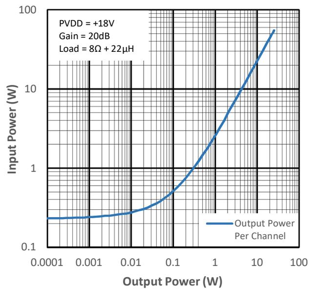
Figure 11-16 Input Power vs Output Power for PMP4
