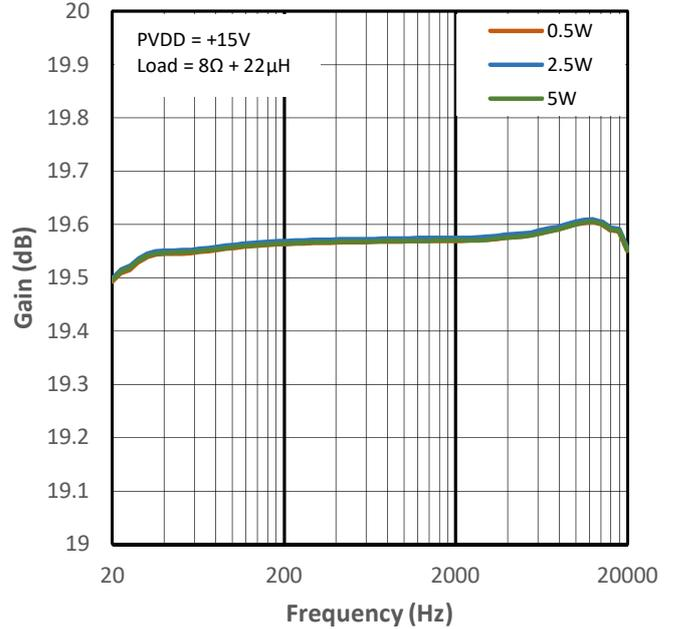
Figure 13-22 Low Gain vs Frequency for PMP1
