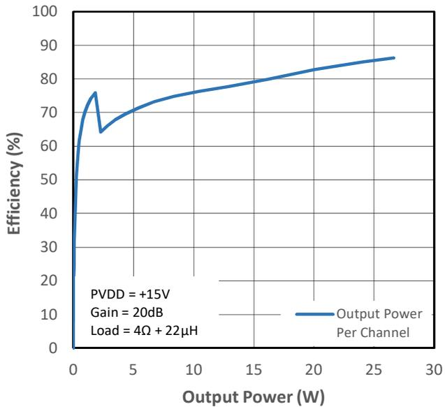
Figure 12-11 PMP2 Efficiency (VDD+PVDD) vs Output Power
