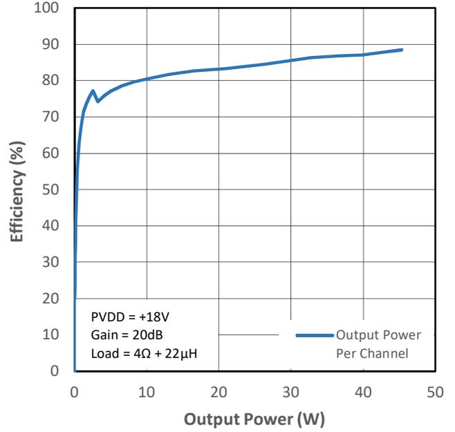
Figure 10-10 PMP1 Efficiency (VDD+PVDD) vs Output Power
