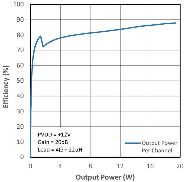
Figure 14-9 PMP0 Efficiency (VDD+PVDD) vs Output Power
