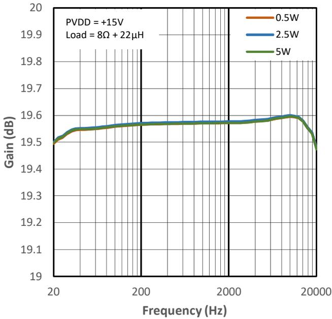
Figure 13-21 Low Gain vs Frequency for PMP0
