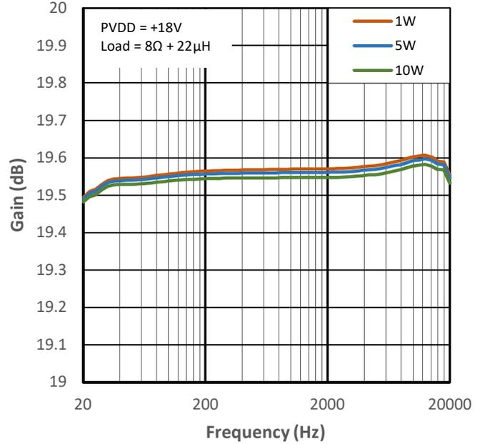
Figure 11-26 Low Gain vs Frequency for PMP1
