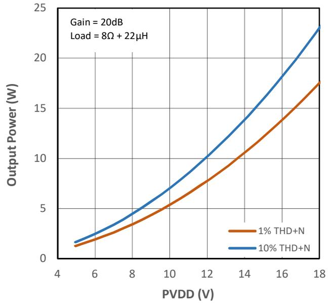
Figure 11-24 Output Power vs PVDD Voltage for PMP4
