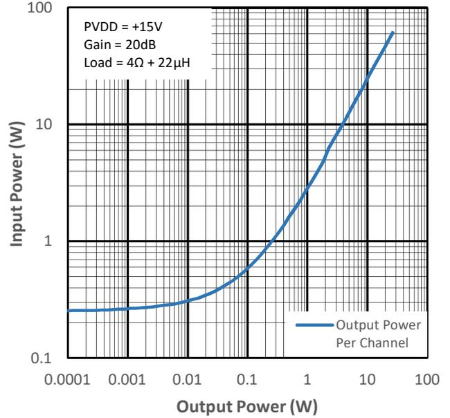
Figure 12-14 Input Power vs Output Power for PMP1
