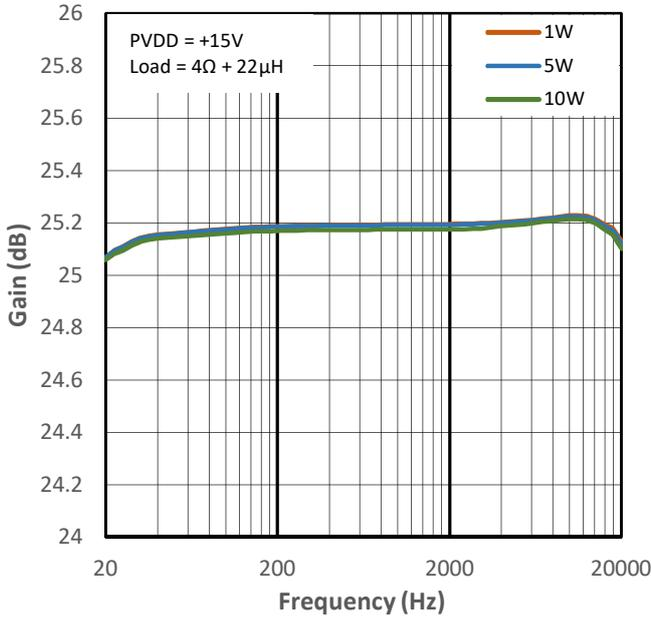
Figure 12-25 High Gain vs Frequency for PMP0
