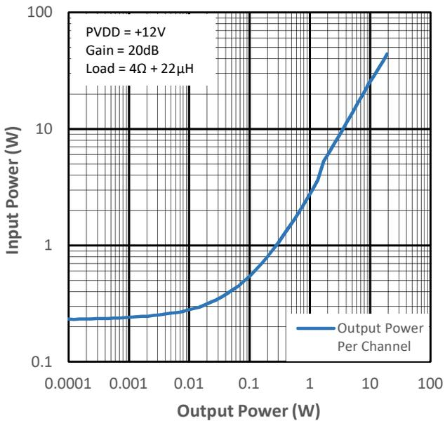
Figure 14-15 Input Power vs Output Power for PMP2
