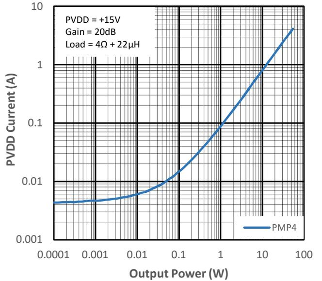
Figure 12-20 PVDD Current vs Output Power for PMP4
