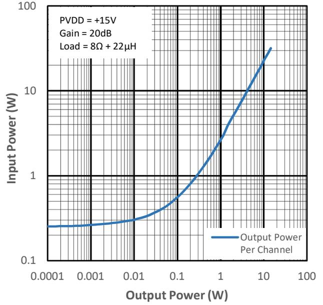
Figure 13-14 Input Power vs Output Power for PMP1
