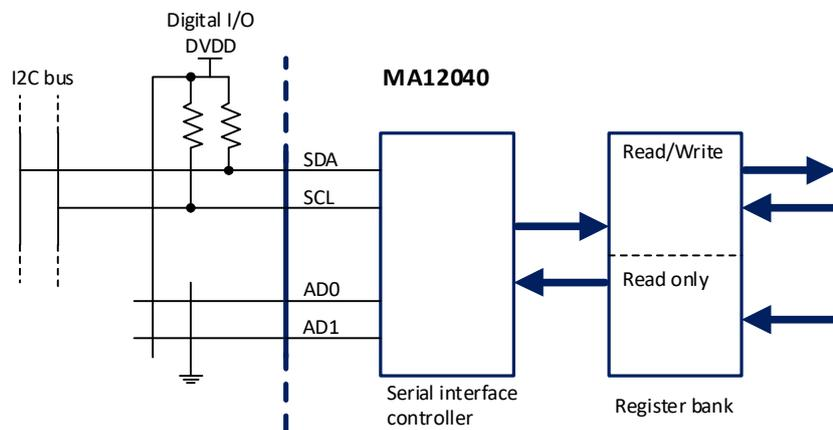
Figure 8-2. I2C bus interface and register bank
