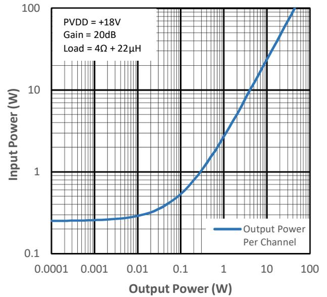
Figure 10-16 Input Power vs Output Power for PMP4
