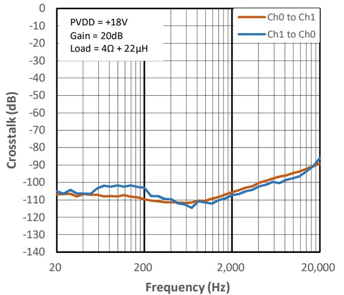
Figure 10-36 Crosstalk vs Frequency for PMP4
