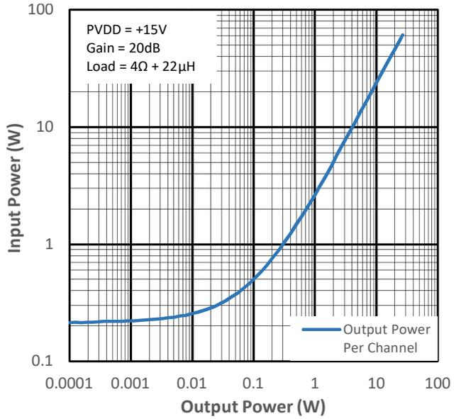
Figure 12-16 Input Power vs Output Power for PMP4
