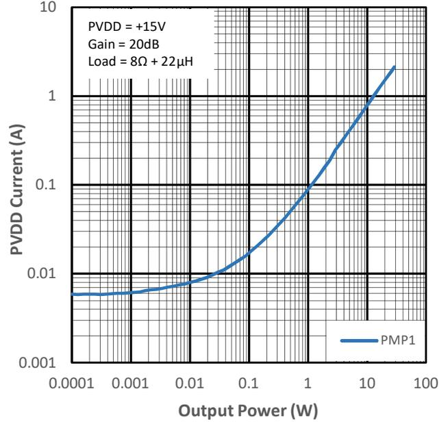
Figure 13-18 PVDD Current vs Output Power for PMP1
