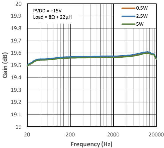
Figure 13-23 Low Gain vs Frequency for PMP2
