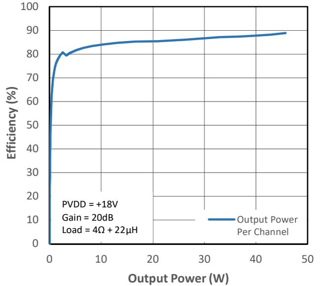
Figure 10-12 PMP4 Efficiency (VDD+PVDD) vs Output Power
