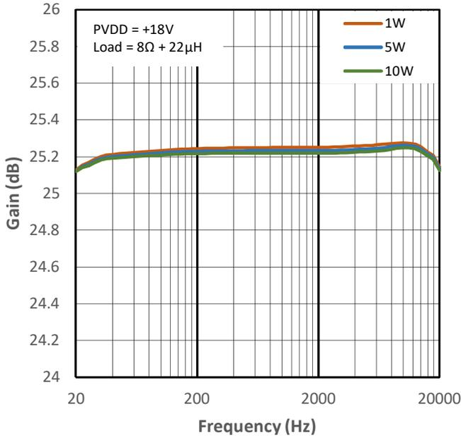
Figure 11-29 High Gain vs Frequency for PMP0
