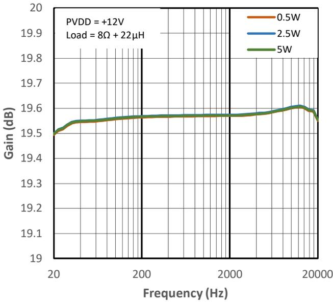
Figure 15-23 Low Gain vs Frequency for PMP2
