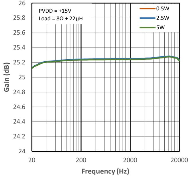
Figure 13-26 High Gain vs Frequency for PMP1
