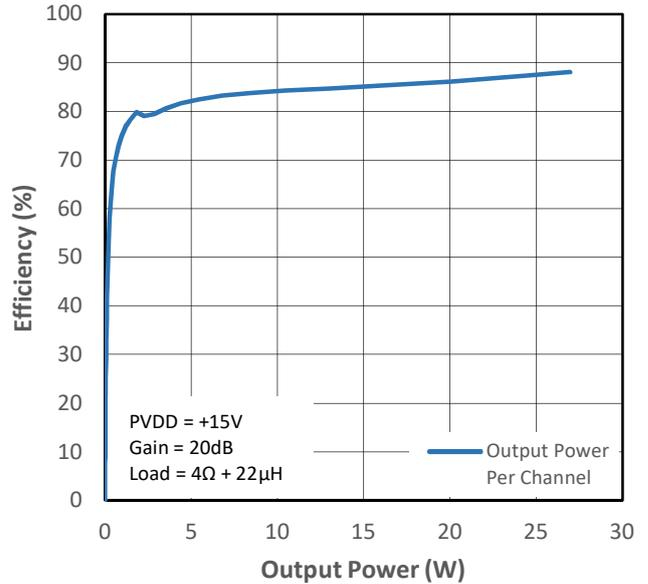
Figure 12-12 PMP4 Efficiency (VDD+PVDD) vs Output Power
