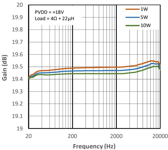
**Figure 10-27 Low Gain vs Frequency for PMP2**
