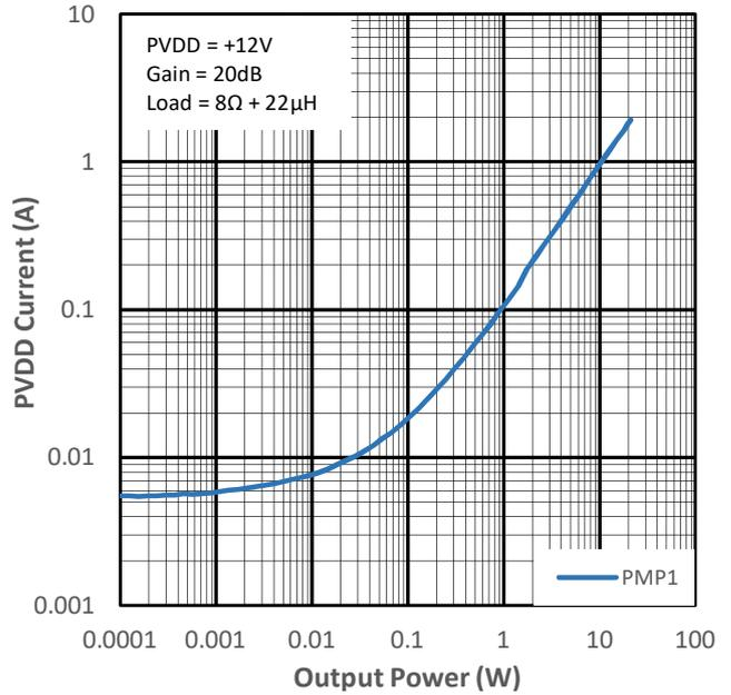
Figure 15-18 PVDD Current vs Output Power for PMP1
