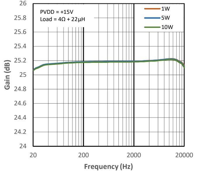
Figure 12-28 High Gain vs Frequency for PMP4
