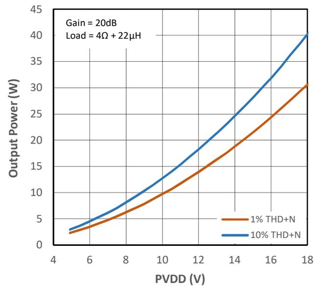
Figure 10-24 Output Power vs PVDD Voltage for PMP4
