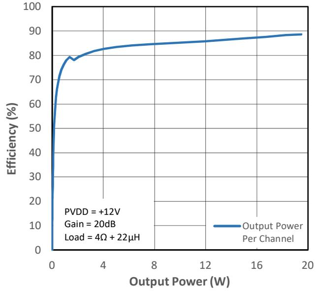
Figure 14-12 PMP4 Efficiency (VDD+PVDD) vs Output Power
