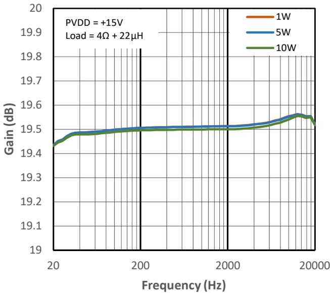
Figure 12-23 Low Gain vs Frequency for PMP2
