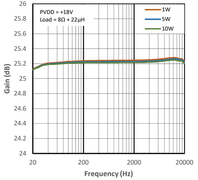
Figure 11-30 High Gain vs Frequency for PMP1
