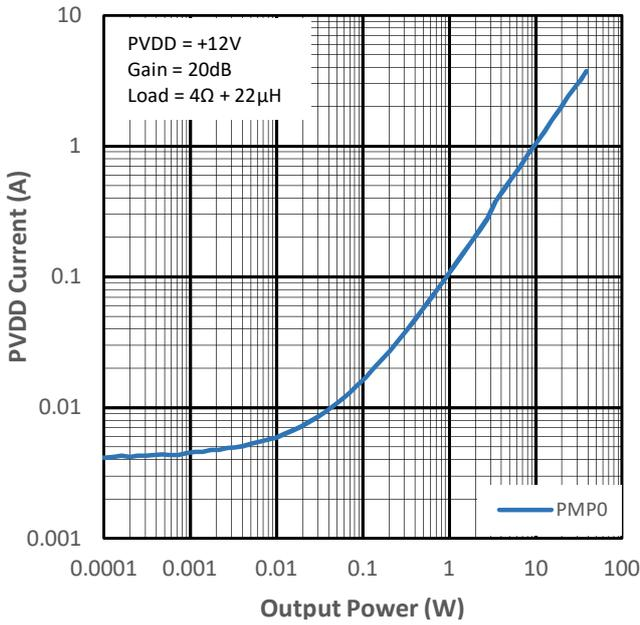
Figure 14-17 PVDD Current vs Output Power for PMP0
