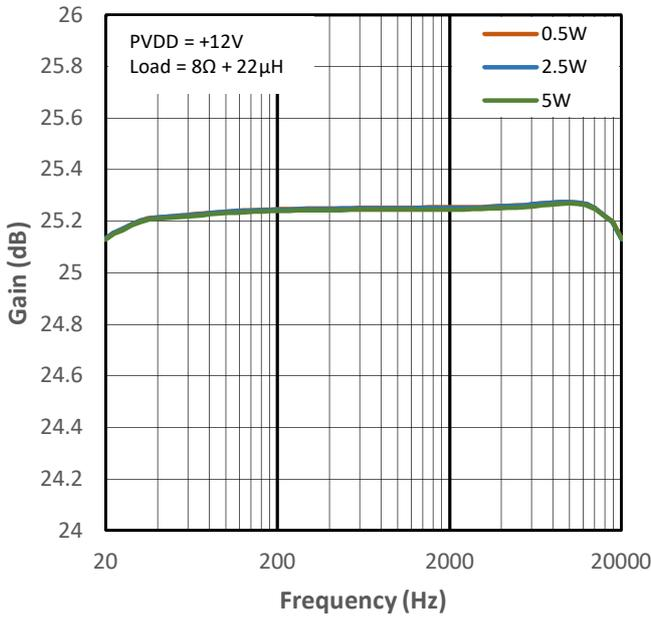
**Figure 15-25 High Gain vs Frequency for PMP0**
