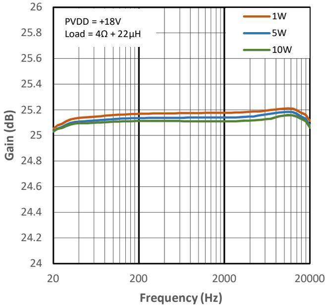
**Figure 10-29 High Gain vs Frequency for PMP0**
