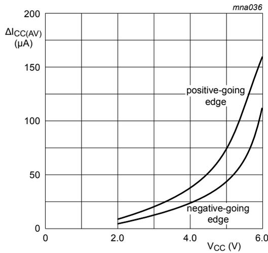
Linear change of  $V_I$  between  $0.1V_{CC}$  to  $0.9V_{CC}$
