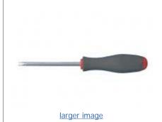
Ergonomically designed handle made from a molded themoplastic rubber which prevents hands from slipping and allows for maximum torque application. Chome-Valadium steel blade with tip hardened to 56-60 HRC.
