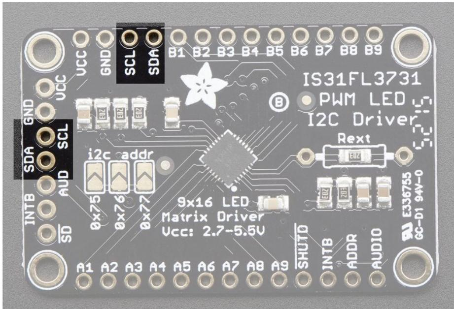
This chip uses I2C for control, it does not use clock stretching or repeated start. There are built in 20K pullups to VCC. You can run it as fast as 400KHz clock speed, but you may need to add additional 2K pullups from SDA and SCL up to VCC for higher speeds
