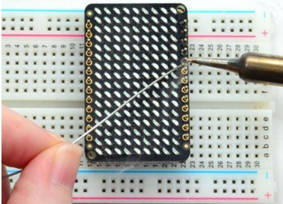
Solder in the two long header strips. Not all are connected on the LED matrix but it makes the connections mechanically stable.
