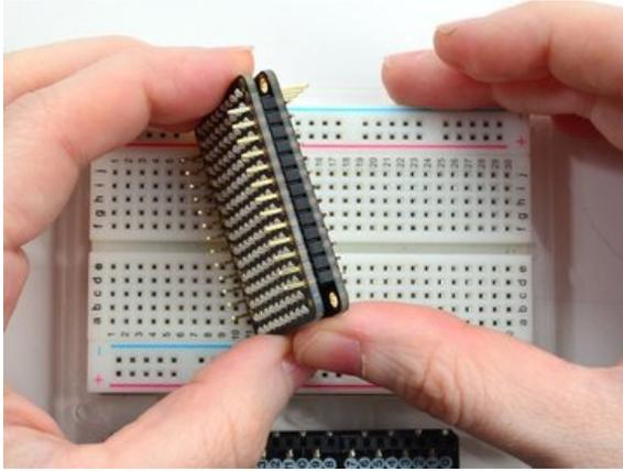
The LEDs face out and connect to the two side header strips.
