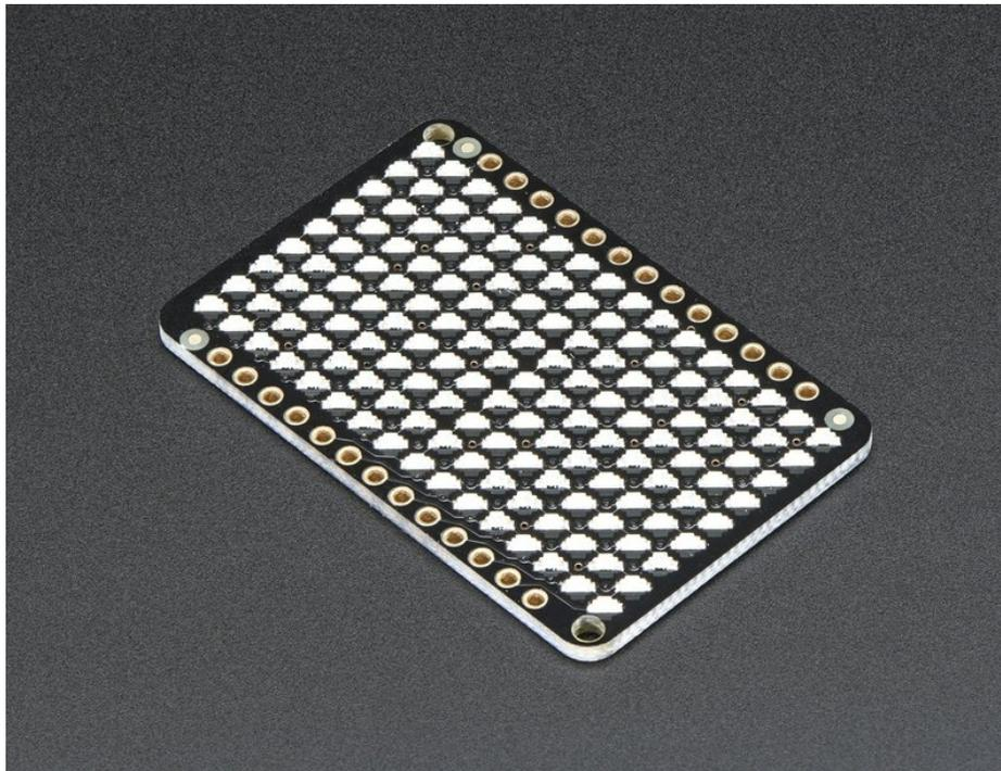
The IS31FL3731 is a nice little chip - it can use 2.7-5.5V power and logic so its flexible for use with any microcontroller. You can set the address so up to 4 matrices can share an I2C bus. Inside is enough RAM
