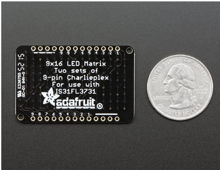
Pick up a driver board and your favorite color LEDs to match. You'll need to do some basic soldering to attach the driver backpack and matrix together, and run wires to your microcontroller, but its not too hard. Then install our Arduino code to get some LEDs blinking immediately. Our library is Adafruit\_GFX
