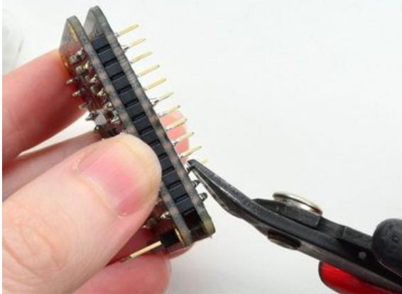
Now you can trim the long header with diagonal cutters. Cut one or two pins at a time
