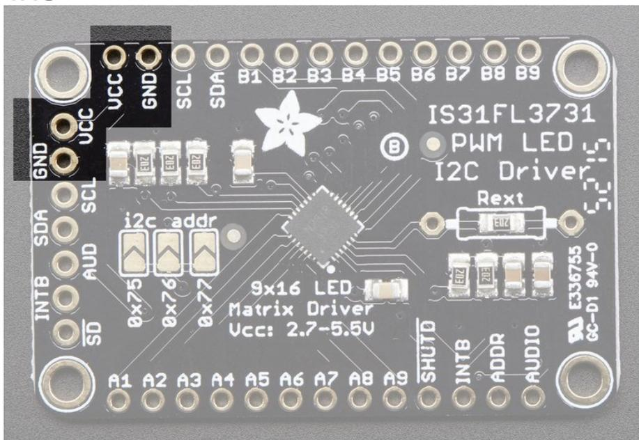
You can power the IS31 from 2.7-5.5VDC, but note that the same voltage is used for both power and logic. If you are using a **5V** logic device, just connect **VCC** to 5V.
