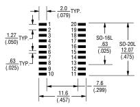
NOTE: Land pattern dimensions are based on design rules established by the Institute for Interconnecting and Packaging Electronic Circuits in IPC-SM-782.
