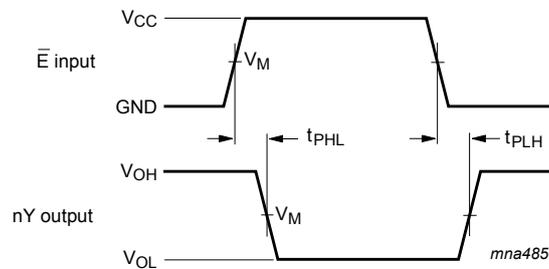
$V_M = 1.5 \text{ V}$  at  $V_{CC} \geq 2.7 \text{ V}$ ;  $V_M = 0.5 \times V_{CC}$  at  $V_{CC} < 2.7 \text{ V}$ .
