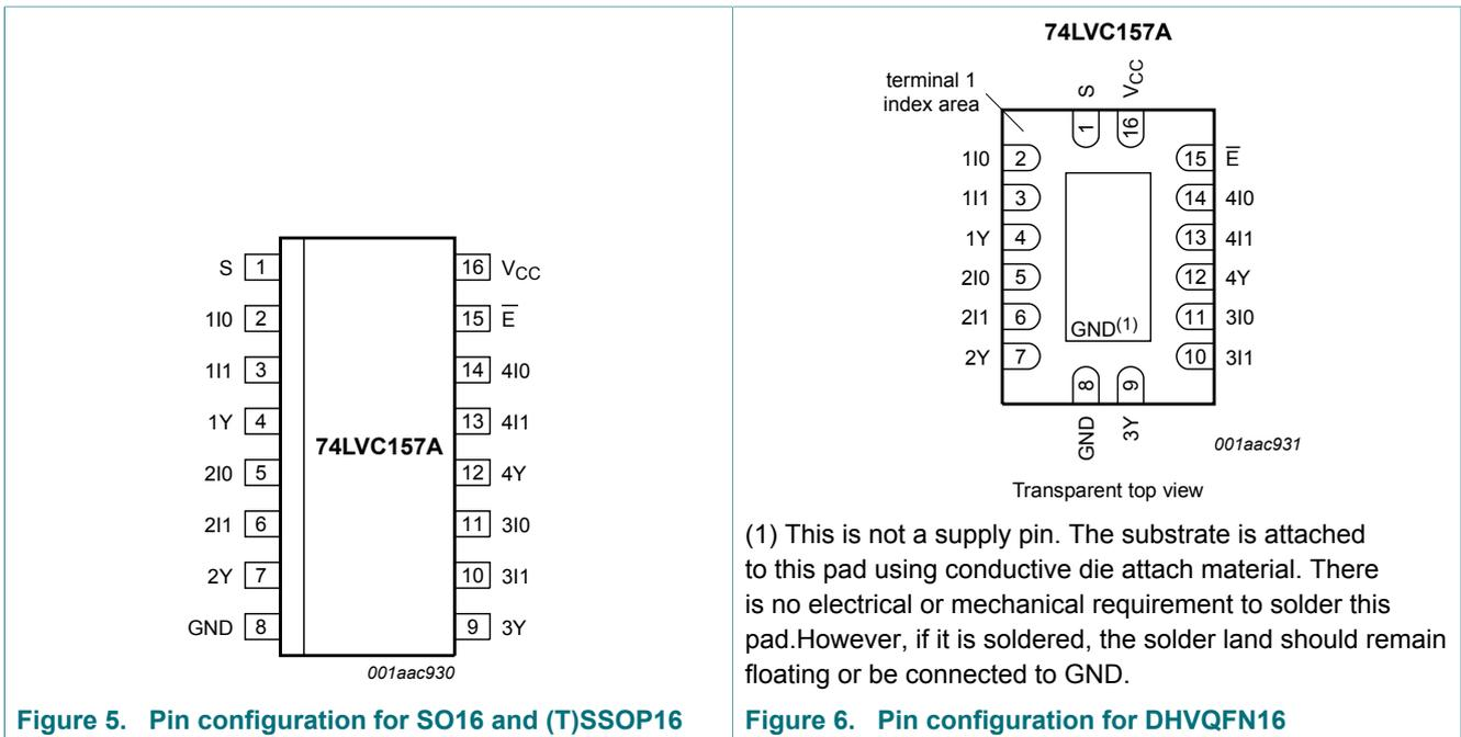
Figure 5. Pin configuration for SO16 and (T)SSOP16
