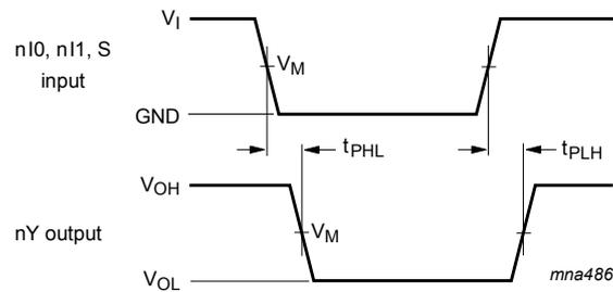
$V_M = 1.5 \text{ V}$  at  $V_{CC} \geq 2.7 \text{ V}$ ;  $V_M = 0.5 \times V_{CC}$  at  $V_{CC} < 2.7 \text{ V}$ .
