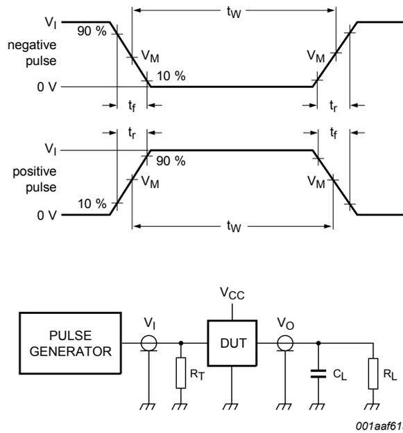
Test data is given in [Table 8](#). Definitions for test circuit:
