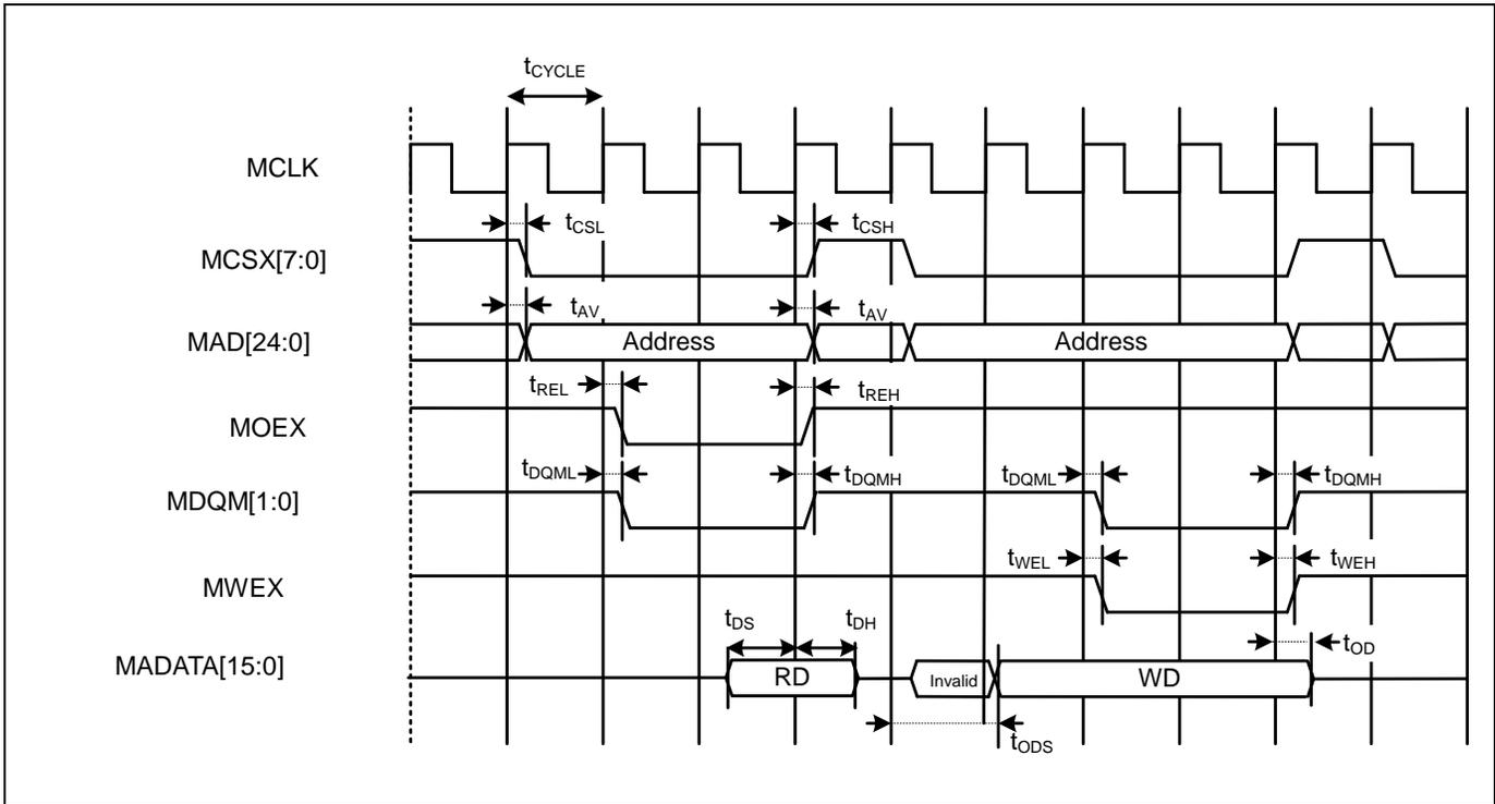
**Multiplexed Bus Access Asynchronous SRAM Mode**
