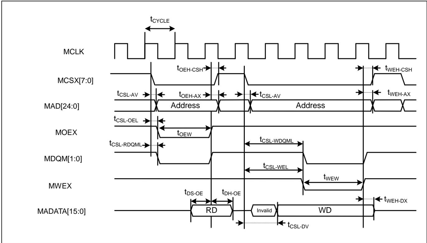
**Separate Bus Access Synchronous SRAM Mode**
