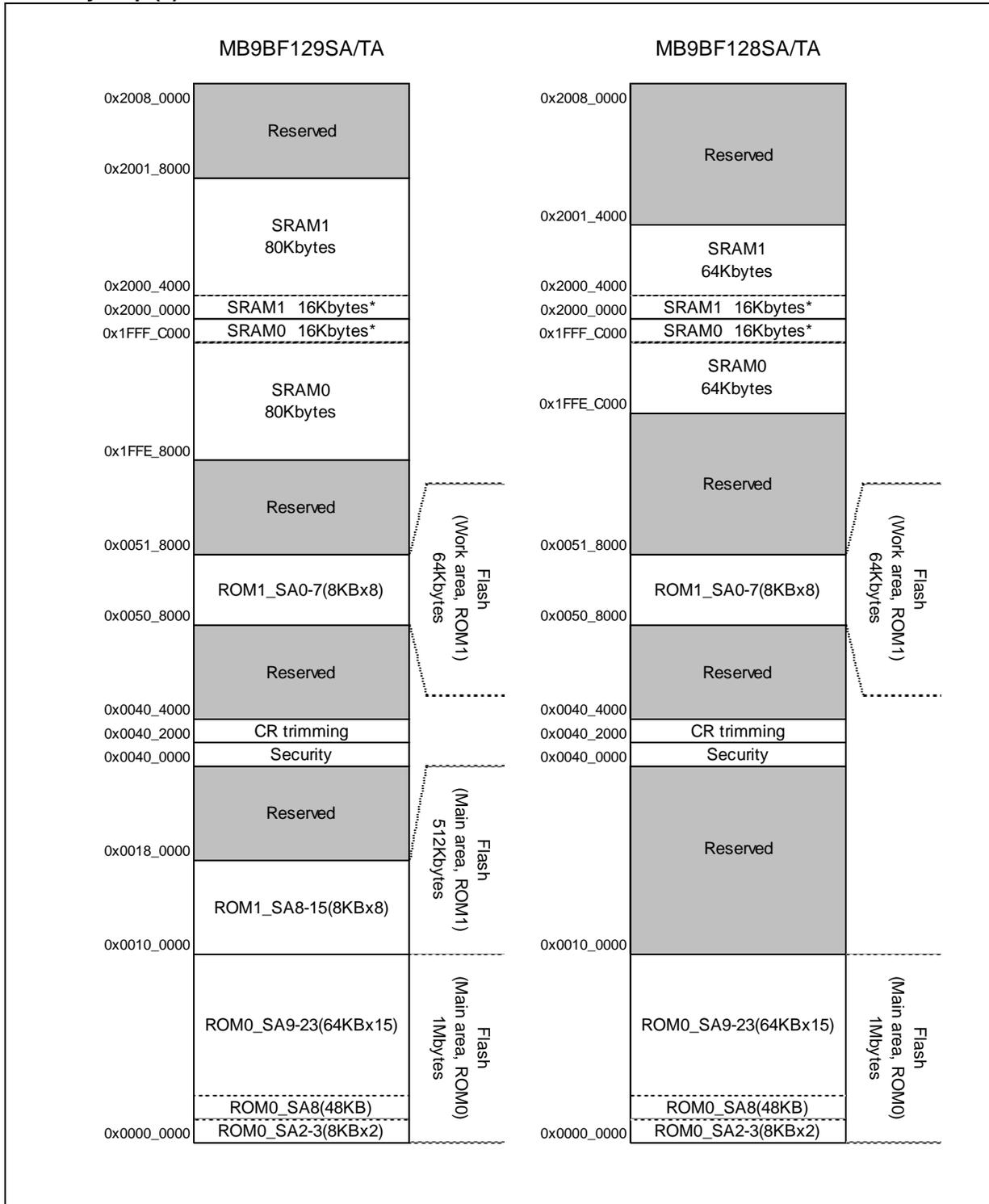
\* : The content of SRAM can be retained at the deep standby modes by the setting of Deep Standby RAM Retention Register (DSRAMR).
