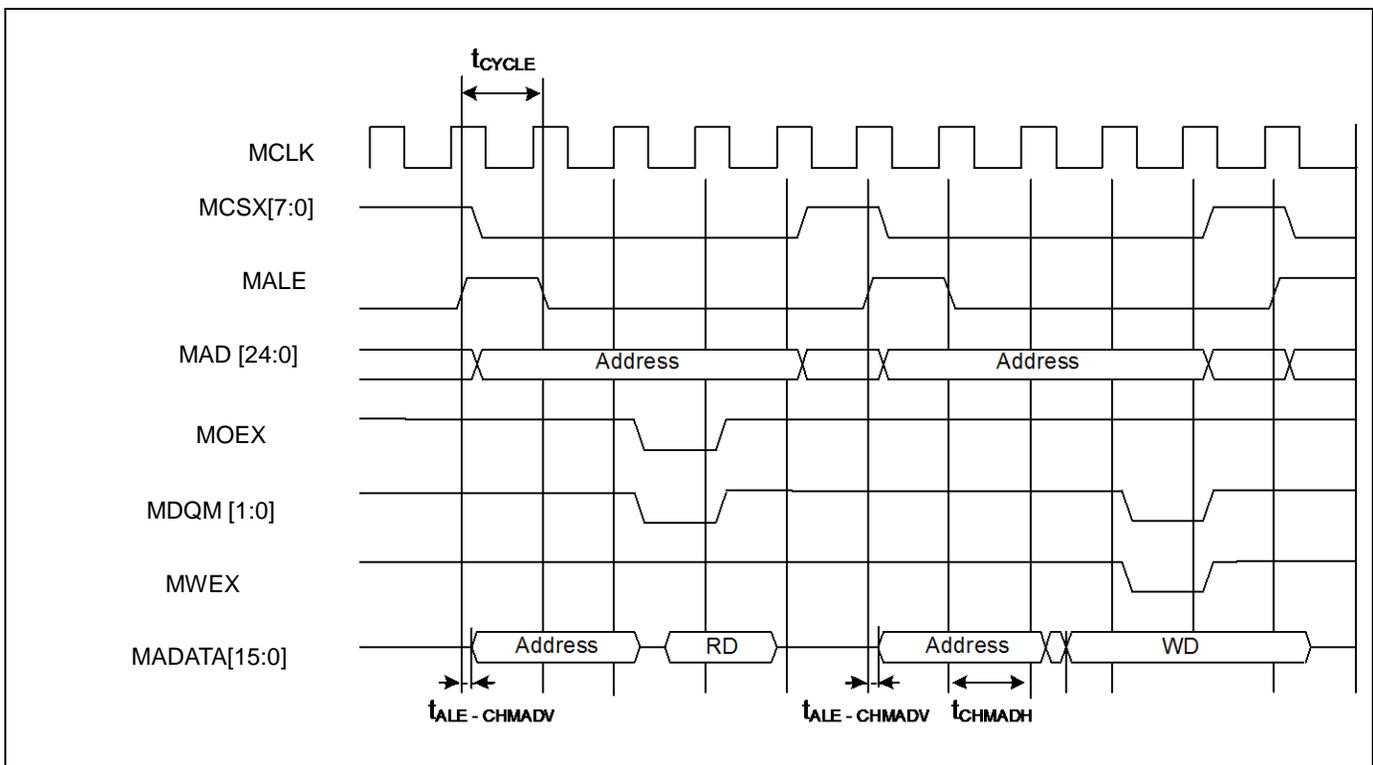
**Multiplexed Bus Access Synchronous SRAM Mode**
