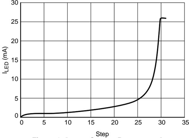
**Figure 4. Output Current Programmed Value ( ILED = F(Step) )**
