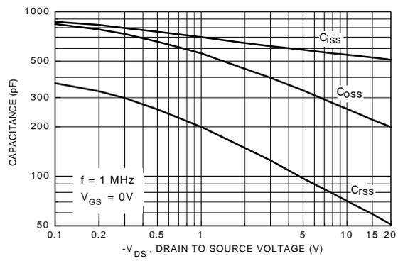
**Figure 9. Capacitance Characteristics.**
