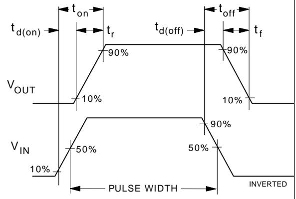
**Figure 12. Switching Waveforms.**
