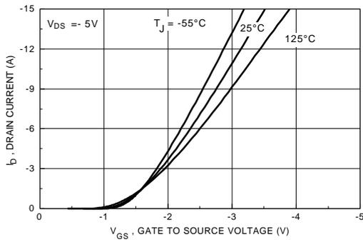
Figure 5. Transfer Characteristics.
