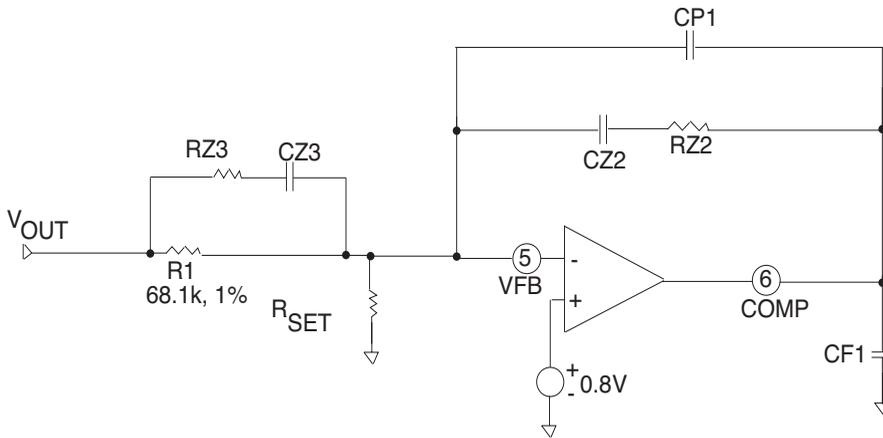
$$R_{SET} = 54.48 / (V_{OUT} - 0.8) \text{ (k}\Omega\text{)}$$
