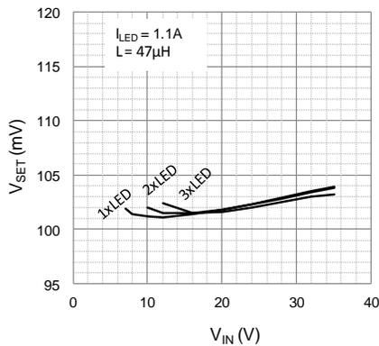
Fig. 8:  $V_{SET}$  versus Input Voltage at  $I_{LED}=1.1A$
