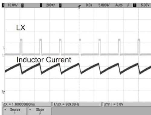
Fig. 12: Switch Waveform
