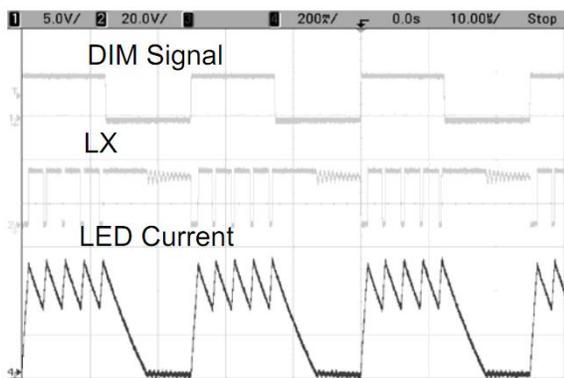
Fig. 14: PWM Dimming
