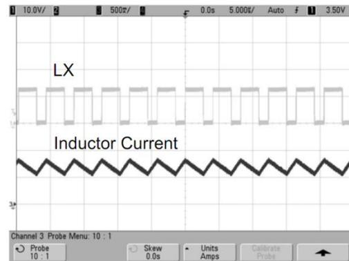
Fig. 13: Switch Waveform
