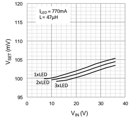
Fig. 7:  $V_{SET}$  versus Input Voltage at  $I_{LED}=770mA$
