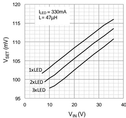
Fig. 6:  $V_{SET}$  versus Input Voltage at  $I_{LED}=330mA$
