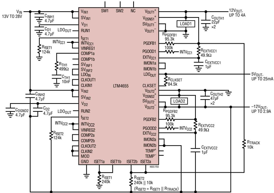
Figure 50. Concurrent ±12V Output DC/DC μModule Regulator
