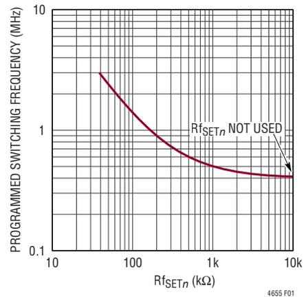
Figure 1. Relationship Between  $R_{fSETn}$  and Target  $f_{SWn}$
