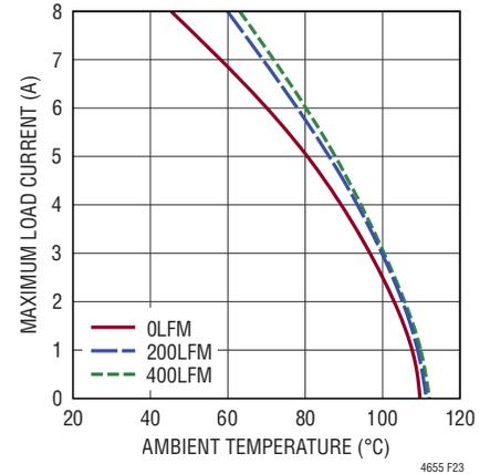
**Figure 22. 24V to 5V<sub>OUT</sub> Derating Curve, with BGA Heat Sink**
