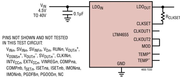
Test Circuit 3. Clock-Generator, 5V LDO and Temperature-Sensor
