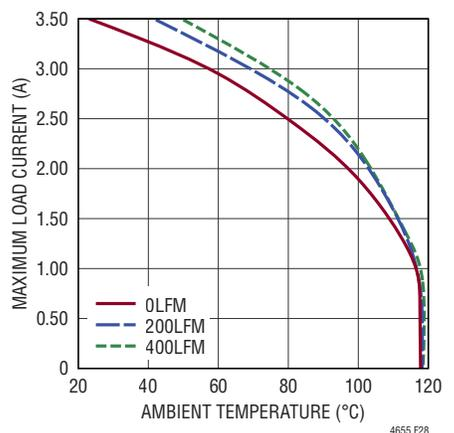
**Figure 28. 5V to -5V<sub>OUT</sub> Derating Curve, No Heat Sink**
