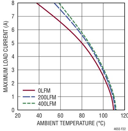
**Figure 21. 12V to 5V<sub>OUT</sub> Derating Curve, with BGA Heat Sink**
