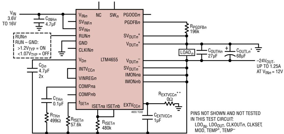
\*Polarized output capacitors  $C_{OUTL}$ , if used, must be rated to withstand  $\sim 0.3V$  typical reverse polarity prior to LTM4655 start-up, stemming from a weakly forward-biased body diode. In such cases, a Schottky diode should be placed local to the LTM4655 and electrically connected between PGND and  $V_{OUTn}^-$  to limit the voltage. See the Applications Information section and Figures 49a and 49b.
