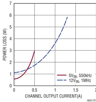
**Figure 27. -24V<sub>OUT</sub> Power Loss Curve**
