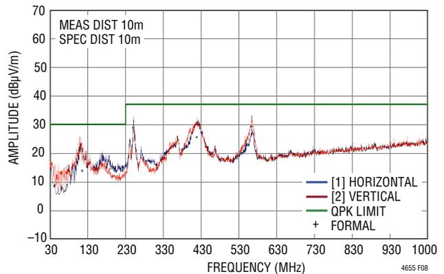
**Figure 8. Radiated Emissions Scan of the LTM4655. Producing -24V<sub>OUT</sub> at 2A, from 12V<sub>IN</sub>, DC2899A Hardware.  $f_{SW} = 1.2\text{MHz}$ . Measured in a 10m Chamber. Peak Detect Method**
