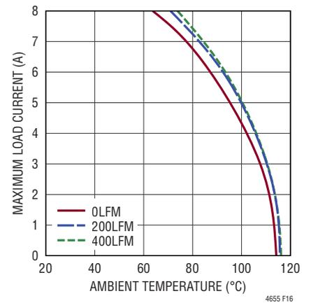
**Figure 16. 5V to 1VOUT Derating Curve, with BGA Heat Sink**
