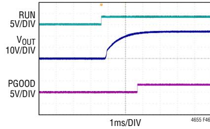
Figure 46. Start-Up Waveforms at 36V<sub>IN</sub>, Figure 45 Circuit
