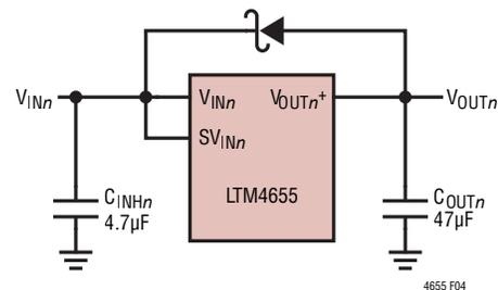
Figure 4. Schottky Diode from  $V_{OUTn}^+$  to  $V_{INn}$
