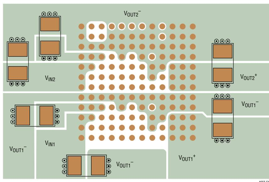
Figure 44. Recommended PCB Layout, Package Top View
