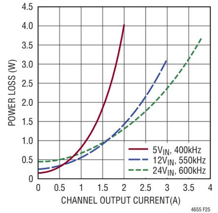
**Figure 25. -5V<sub>OUT</sub> Power Loss Curve**
