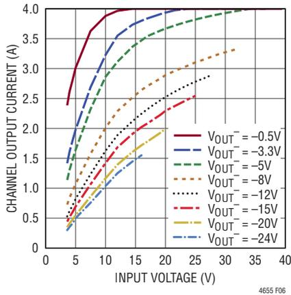
**Figure 6. Channel Output Current Capability\*, Negative- $V_{OUT}$  Operation**
