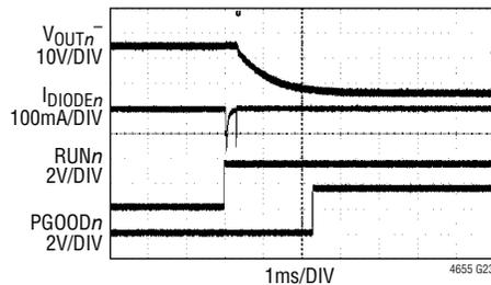
FIGURE 48 CIRCUIT,  $V_{OUTn^-}$  PRE-BIASED
