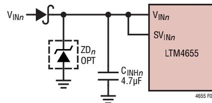
Figure 3. Schottky Diode in Series with the Supply
