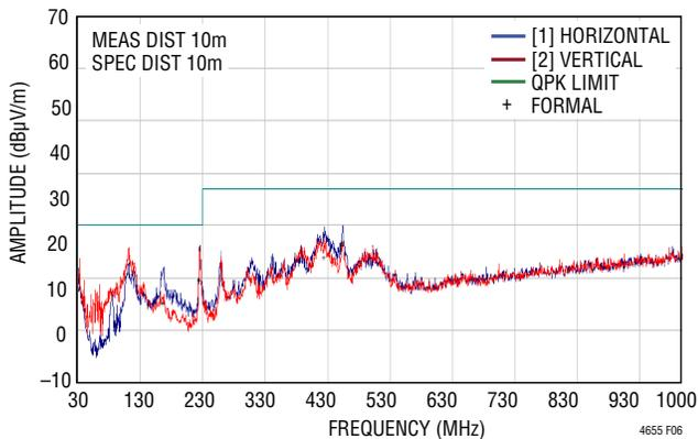
**Figure 7. Radiated Emissions Scan of the LTM4655. Producing 24V<sub>OUT</sub> at 7A, from 36V<sub>IN</sub>. DC2898A Hardware.  $f_{SW} = 1.2\text{MHz}$ . Measured in a 10m Chamber. Peak Detect Method**
