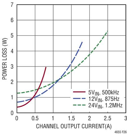
**Figure 26. -15V<sub>OUT</sub> Power Loss Curve**
