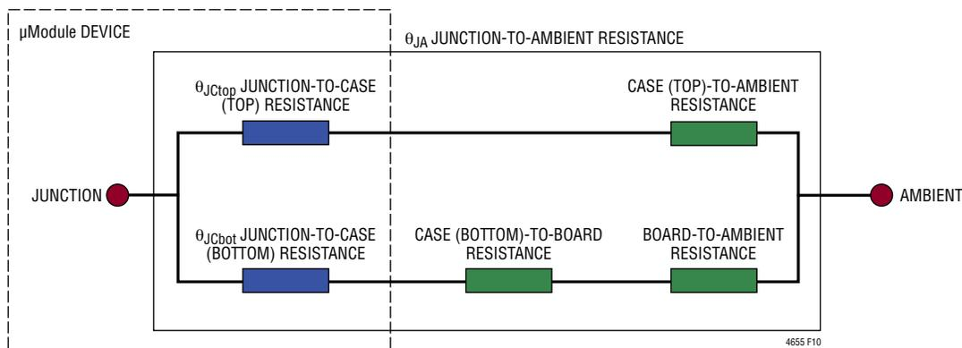
Figure 10. Graphical Representation of JEDEC Thermal Coefficients
