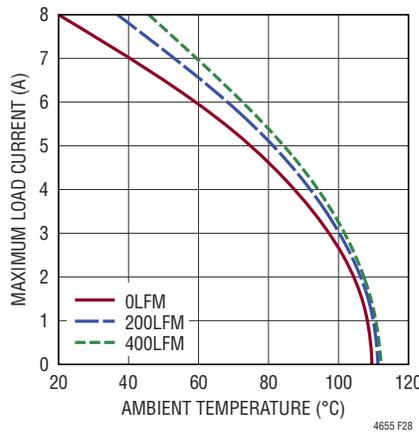
**Figure 24. 24V to 15V<sub>OUT</sub> Derating Curve, with BGA Heat Sink**
