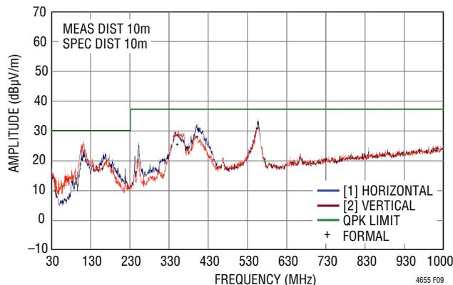
**Figure 9. Radiated Emissions Scan of the LTM4655. Producing -12V<sub>OUT</sub> at 4A, from 12V<sub>IN</sub>. DC2899A Hardware.  $f_{SW} = 700\text{kHz}$ . Measured in a 10m Chamber. Peak Detect Method**
