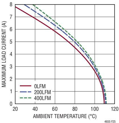
**Figure 23. 24V to 15V<sub>OUT</sub> Derating Curve, No Heat Sink**
