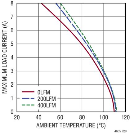
**Figure 20. 24V to 5V<sub>OUT</sub> Derating Curve, No Heat Sink**
