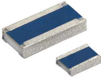
NCW AT low ohmic resistors are the perfect choice for most fields of modern professional power measurement electronics where reliability, stability, power dissipation and robust design is of major concern. The product features extraordinary temperature cycling robustness, verified through extensive testing. The permissible power rating is specified with up to 1 W for size 0612. Typical applications are current measurements in power electronics within automotive and industrial appliances.
