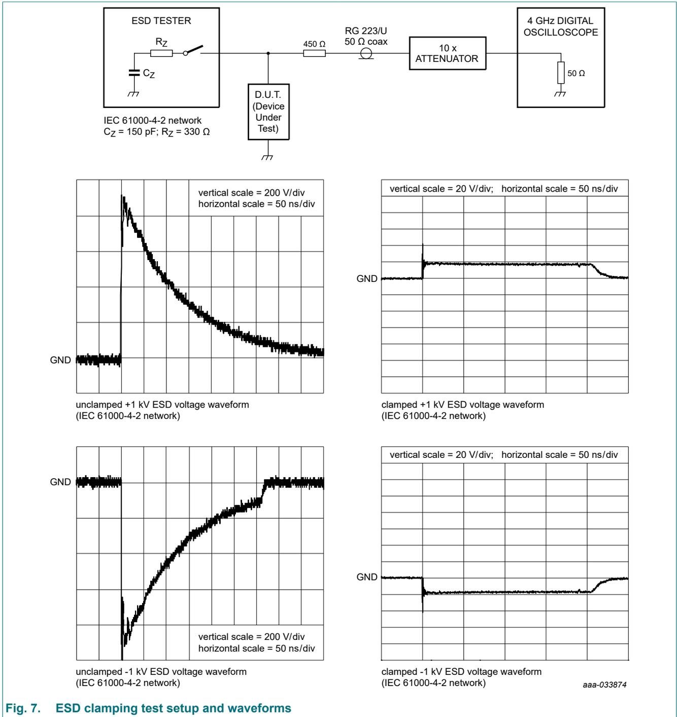
Fig. 7. ESD clamping test setup and waveforms
