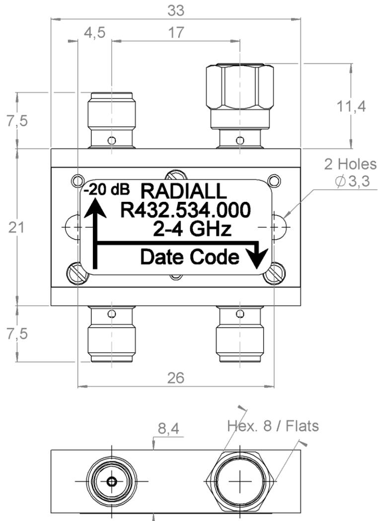
All dimensions are in mm. Tolerances according ISO 2768 m-H
