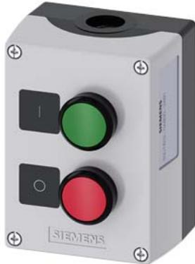
Enclosure for command devices, 22 mm, round, Enclosure material plastic, enclosure top part gray, 2 control points plastic, B=Pushbutton green, label: I, 1 NO, screw terminal, A=Pushbutton red, label: O, 1 NC, screw terminal, floor mounting, 1xM20 each on top and bottom, Labels enclosed
