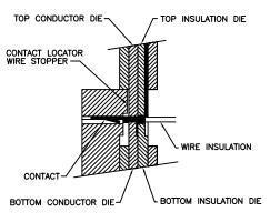
SECTION THROUGH DIE NEST WITH CONTACT IN POSITION
