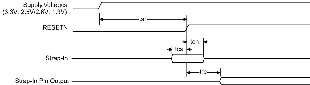
Figure 16. Reset Timing
