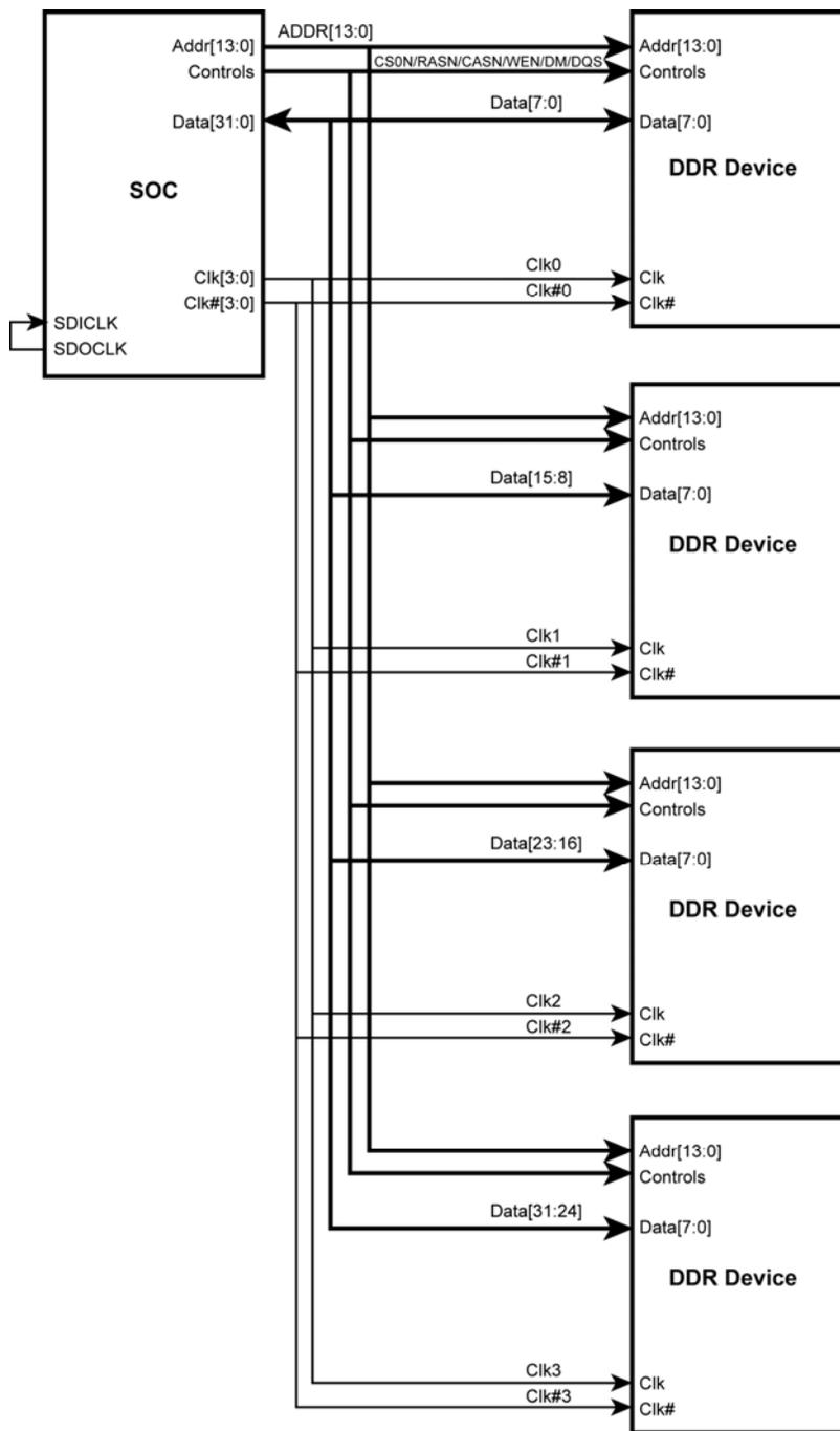
Figure 9. Four8-bit DDR Memory Devices Interface Example
