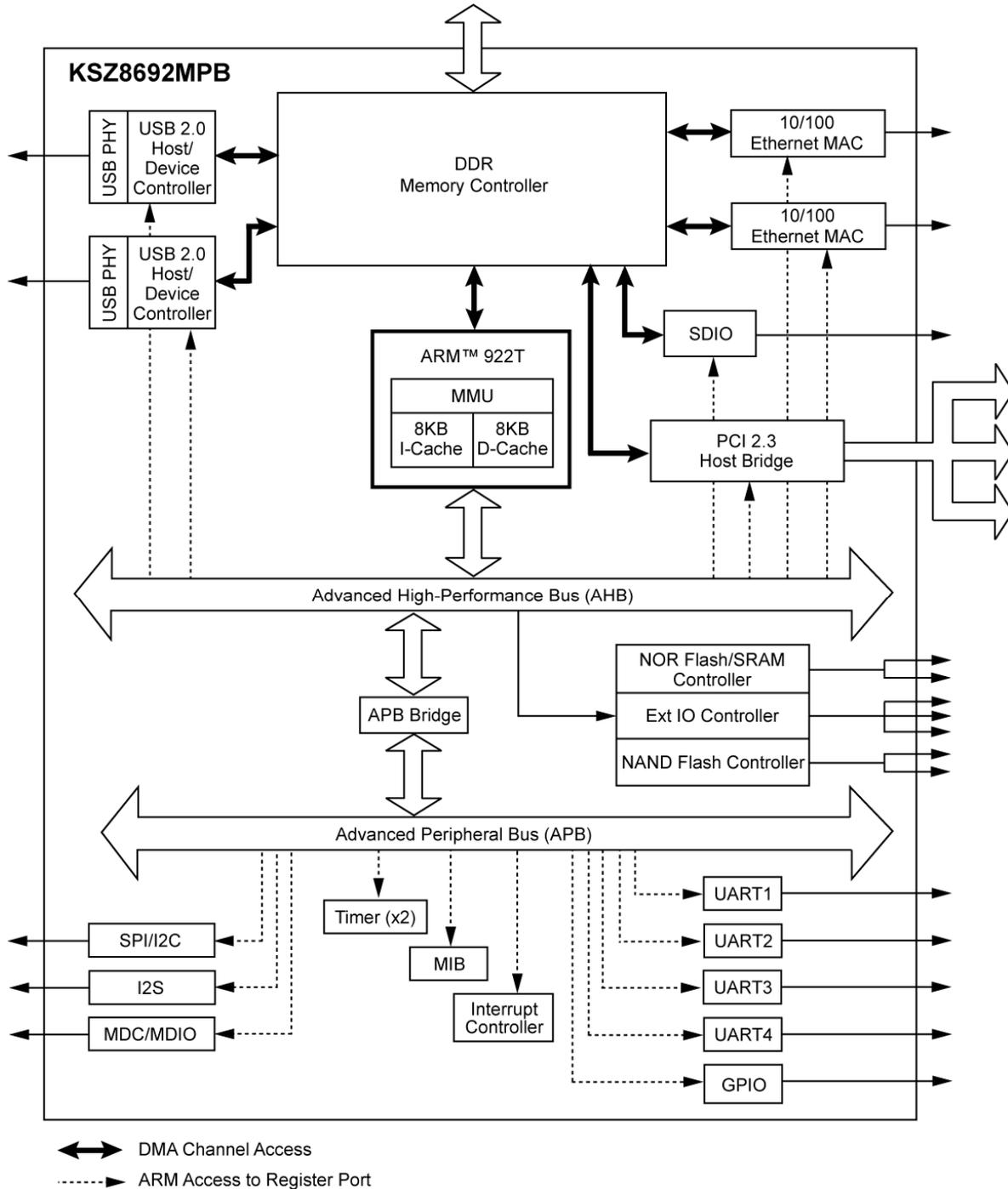
Figure 3. KSZ8692MPB Functional Block Diagram
