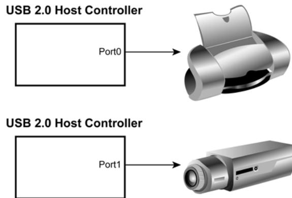
Figure 12. USB 2.0 Configuration as Two-Port Host
