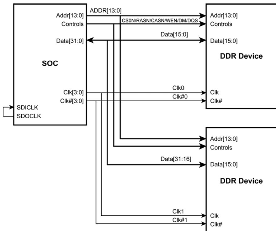
Figure 8. Two 16-bit DDR Memory Device Interface Example
