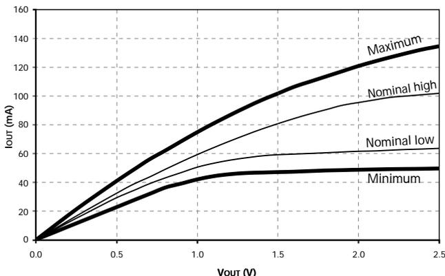
Figure 10: Pull-Up Characteristics
