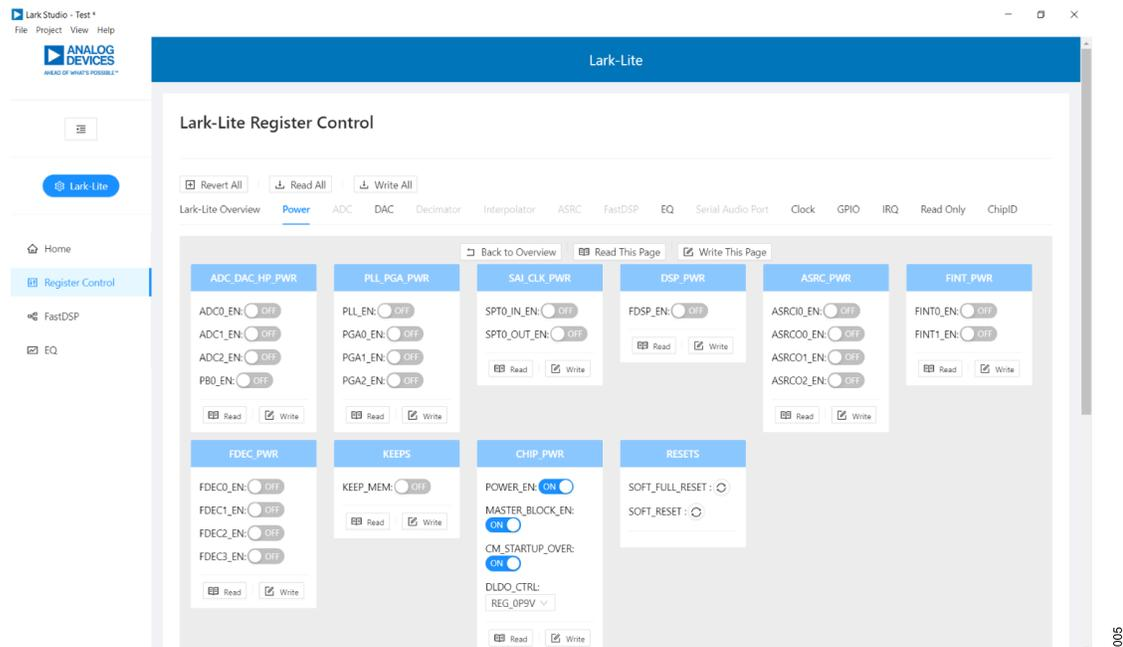
Figure 5. Register Configuration
