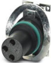
Flush-type connector, 3-position, SocketLink:straightLink:M8, A-coded, PCB mounting, SMD
