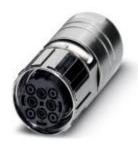
Cable connector, straight short, Screw locking, M40, number of positions: 4+3+PE, type of contact: Socket, Crimp connection, shielded: yes, cable diameter range: 21 mm ... 25.5 mm
