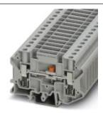
Test disconnect terminal block, Connection method: Screw connection with spring support, Cross section: 0.2 mm² -10 mm², AWG: 24 - 10, Width: 8.2 mm, Mounting type: NS 35/7,5, NS 35/15, NS 32, Color: gray
