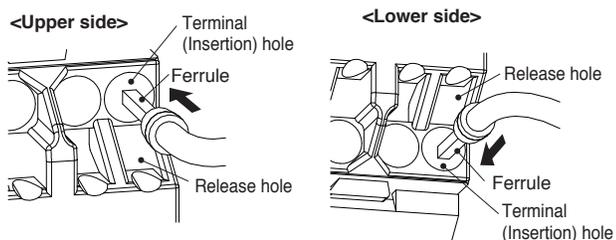
If a wire is difficult to connect because it is too thin, use a flat-blade screwdriver in the same way as when connecting stranded wire.
