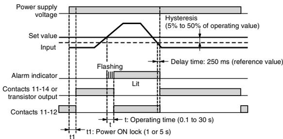
Note: The power ON lock prevents unnecessary alarms from being generated during the instable period when the power is first turned on. There is no relay output during timer operation.
