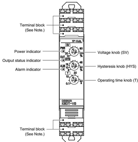
**Note:** Use stranded wires with or without ferrules to connect to the terminals.
