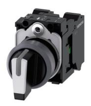
Selector switch, illuminable, 22 mm, round, plastic with metal front ring, white, selector switch, short, 3 switch positions I-O-II, latching, actuating angle  $2x45^{\circ}$ , 10:30h/12h/13:30h, with holder, 1 NO, 1 NO, spring-type terminal, Z=20-unit packaging
