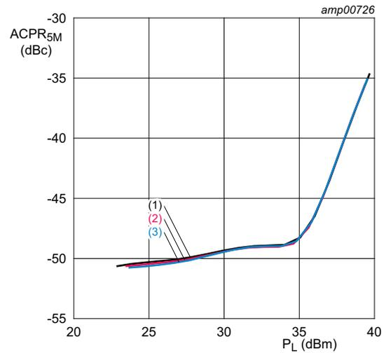
$V_{DS} = 50\text{ V}; I_{Dq} = 100\text{ mA}.$
