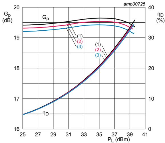
$V_{DS} = 50\text{ V}; I_{Dq} = 100\text{ mA}.$
